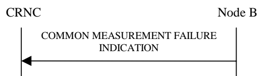
Figure 15: Common Measurement Failure procedure, Successful Operation
