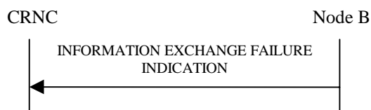
Figure 27P: Information Exchange Failure procedure, Successful Operation
