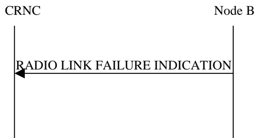
Figure 43: Radio Link Failure procedure, Successful Operation
