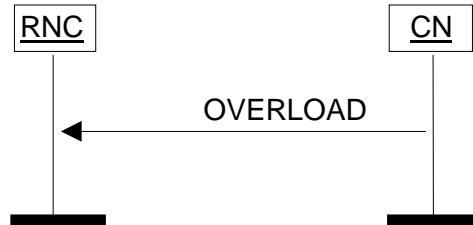
Figure 144: Overload at the CN. Successful operation.
