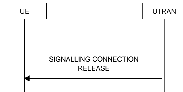
Figure 19: Signalling connection release procedure, normal case
