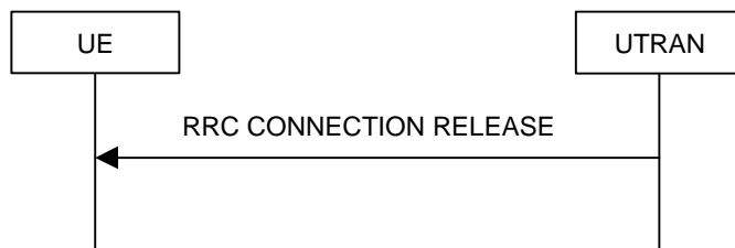
Figure 11: RRC Connection Release procedure on the CCCH
