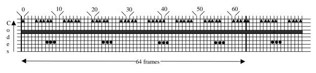
hysic. channel (Code 7; Repetition period=8; Repetition length=5; Activation time =  $4 \Rightarrow \text{Offset} = 4 \Rightarrow \text{CFN}_{\text{off}} = 4, 12, 20, 28, 36, 44, 52, 60$ )
