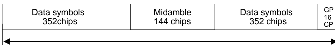
Figure 2 Burst structure for normal traffic time slot
