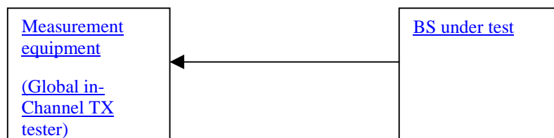
Figure B.2: Measurement system setup for RF frequency, several code power tests and transmit modulation (EVM and PCDE)
