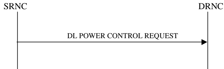
Figure 5: Downlink Power Control procedure, Successful Operation
