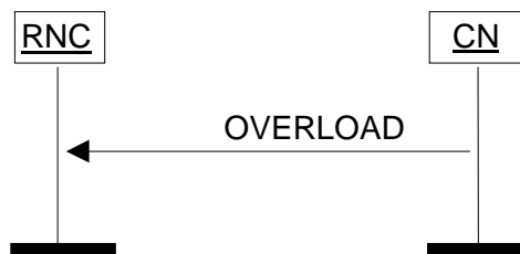
Figure 29: Overload at the CN
