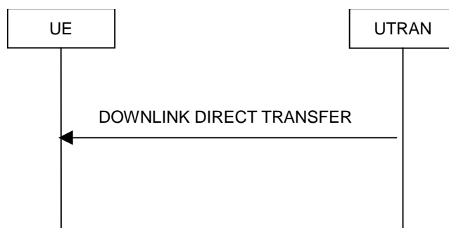
Figure 15: Downlink Direct transfer, normal flow
