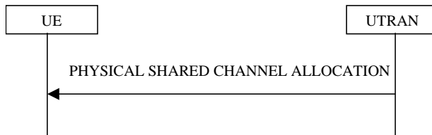
Figure 34: Physical Shared Channel Allocation
