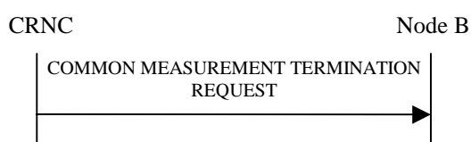
Figure 14: Common Measurement Termination procedure: Successful Operation
