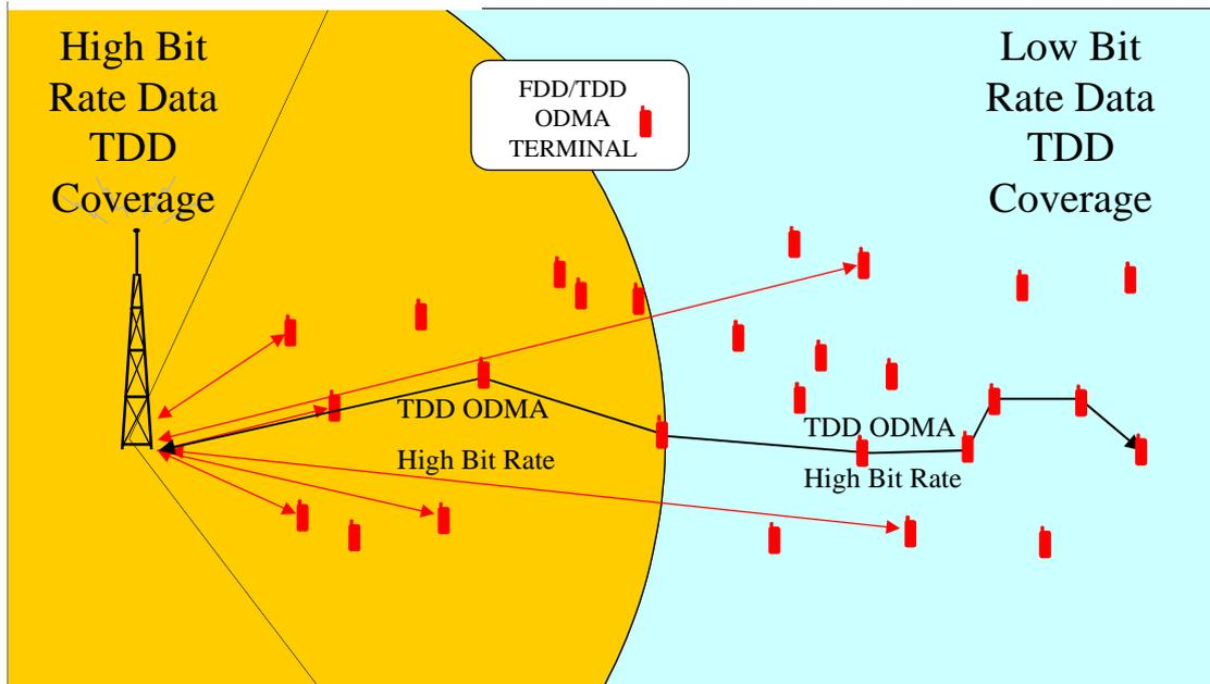
Figure 2: ODMA concept diagram with integrated TDD/ODMA NodeB
