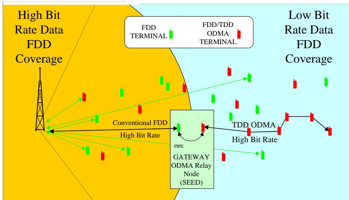
Figure 3: ODMA concept diagram with last hop
