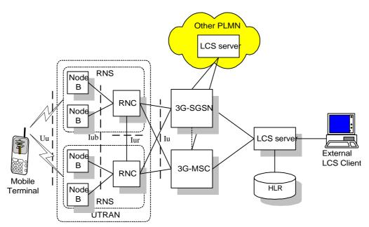
Figure 5.1, General arrangement of LCS in UMTS
