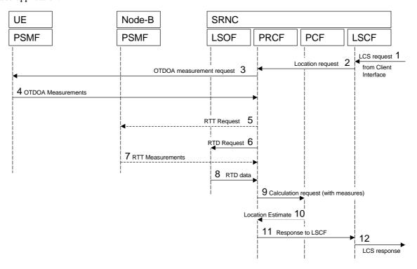
**Figure – OTDOA Signalling Operations**
