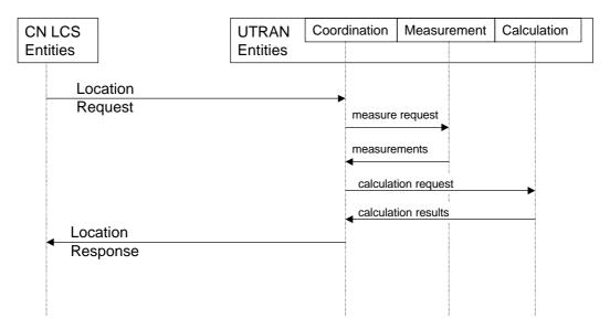
Figure 5.2, General sequence for LCS operation
