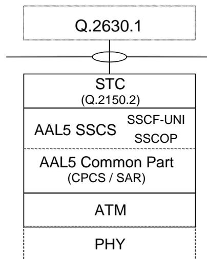
**Figure 2:** Transport Network Control plane protocol structure on I<sub>ub</sub>.
