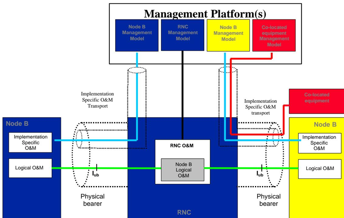
**Figure Error! Unknown switch argument.: Implementation Specific O&M Transport via RNC**
