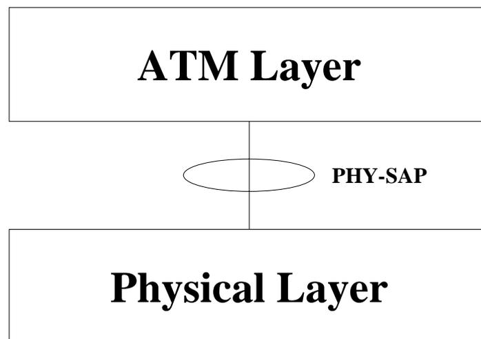
**Figure 1: SAP between Physical Layer and ATM Layer**
