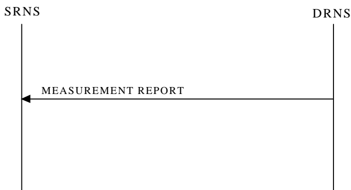
Figure 7-7. Radio Measurements Reporting
