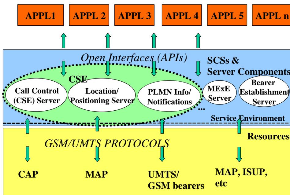
The Service Capability Servers reflect the service capabilities in UMTS phase1, i.e. access to bearers, CAMEL, MExE and SIM-Toolkit. The functionality of these can further be subdivided into server components dedicated to specific tasks.
