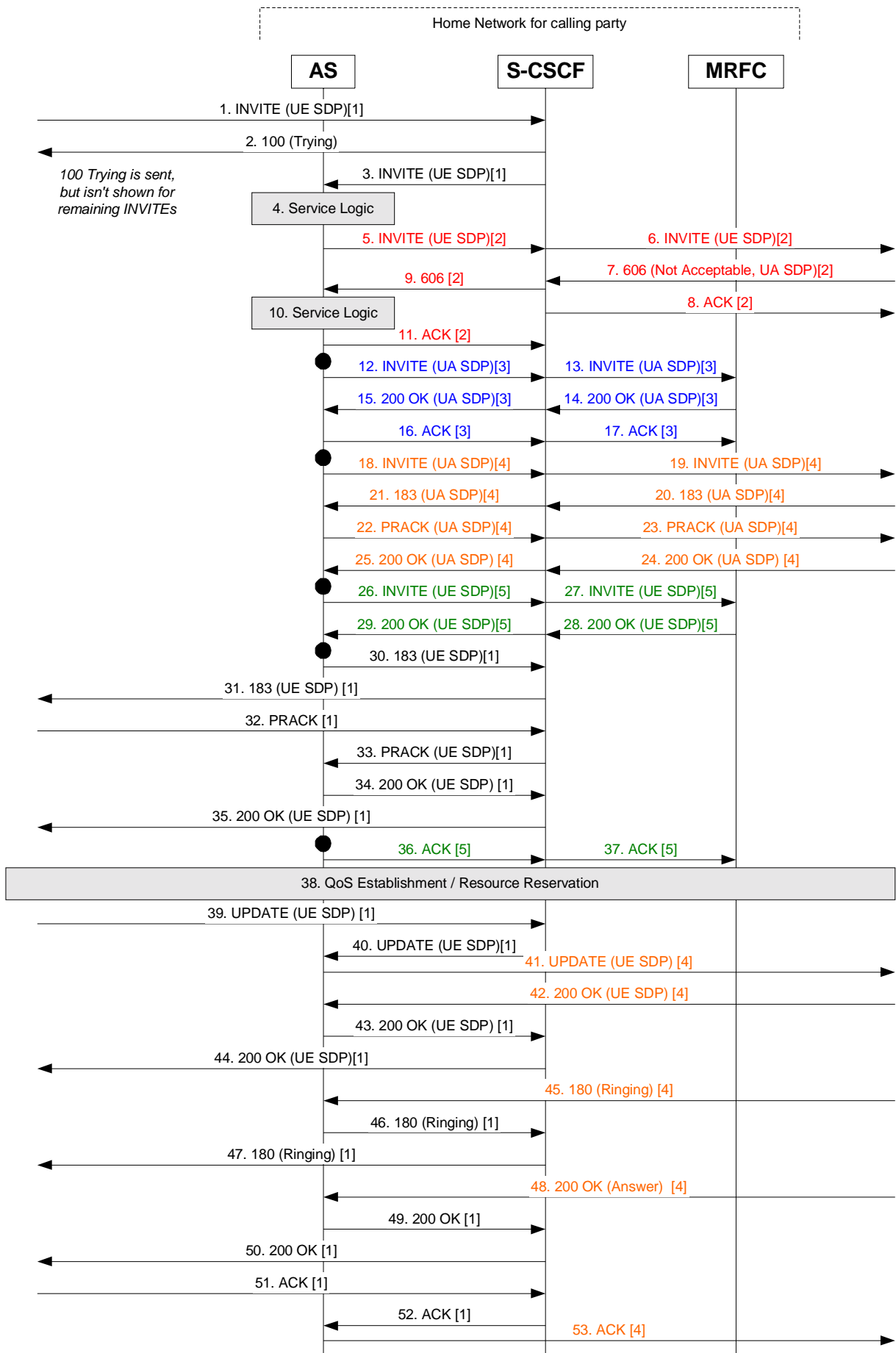
Figure B.2.3.1: Transcoding call flow (called party indicates codec)
