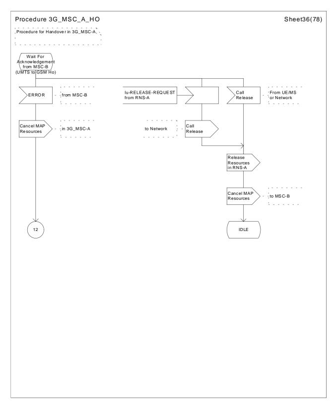
Figure 43 (sheet 36 of 78): Handover control procedure in 3G\_MSC-A
