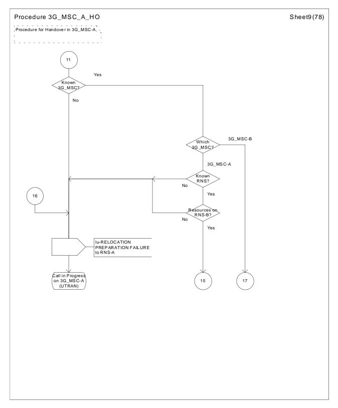
Figure 43 (sheet 9 of 78): Handover control procedure in 3G\_MSC-A
