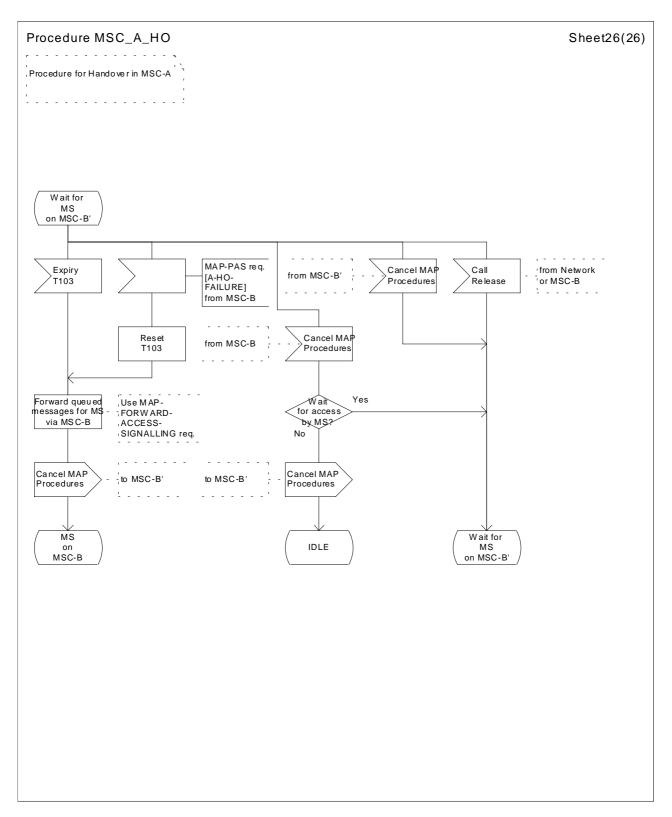
Figure 41 (Sheet 26 of 26): Handover control procedure in MSC-A
