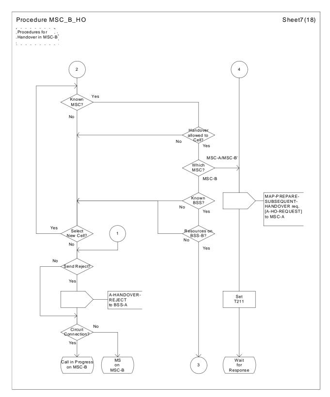
Figure 42 (Sheet 7 of 18): Handover control procedure in MSC-B
