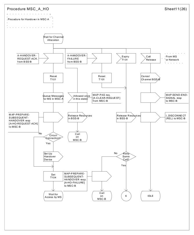
Figure 41 (Sheet 11 of 26): Handover control procedure in MSC-A
