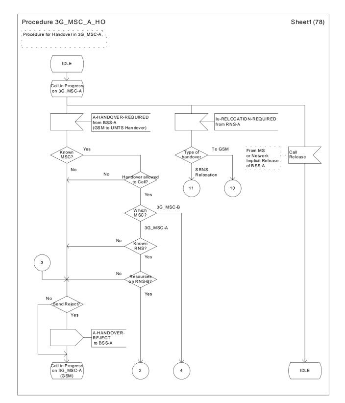
Figure 43 (sheet 1 of 78): Handover control procedure in 3G\_MSC-A
