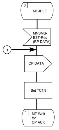
MT-SMC-GP entity on Network-side for GPRS SDL-22
