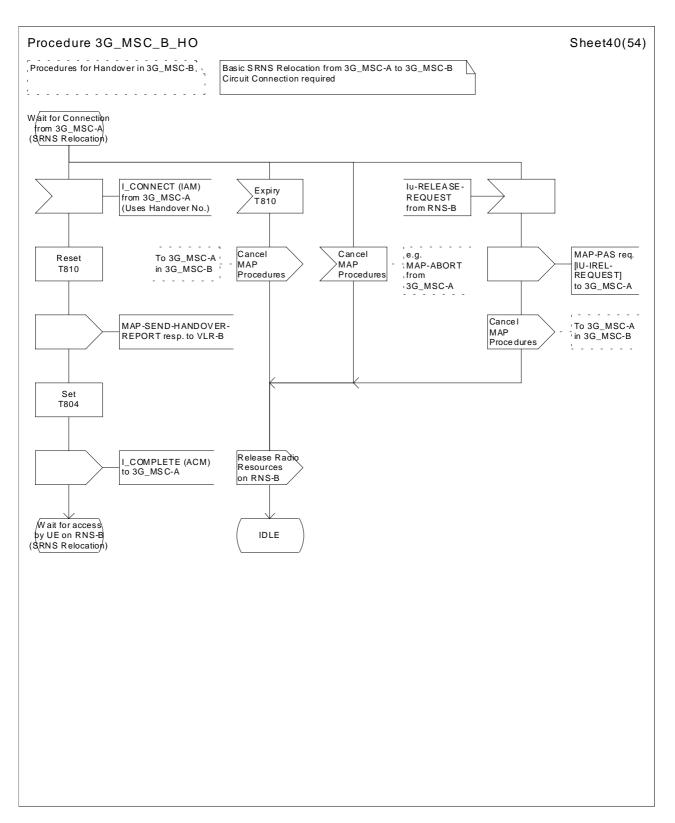
Figure 44 (sheet 40 of 54): Handover control procedure in 3G\_MSC-B
