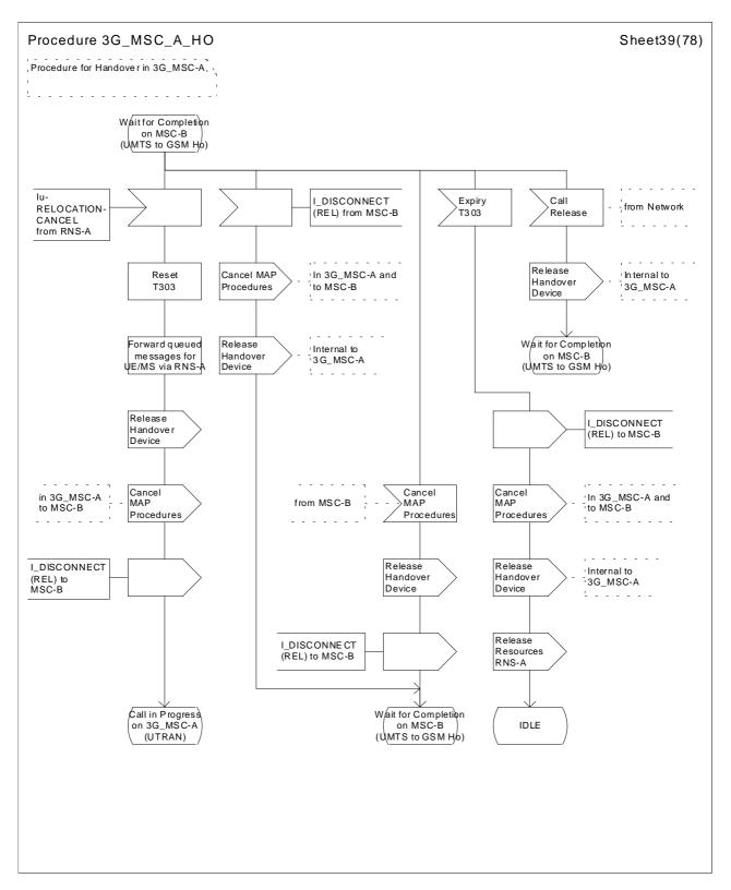
Figure 43 (sheet 39 of 78): Handover control procedure in 3G\_MSC-A
