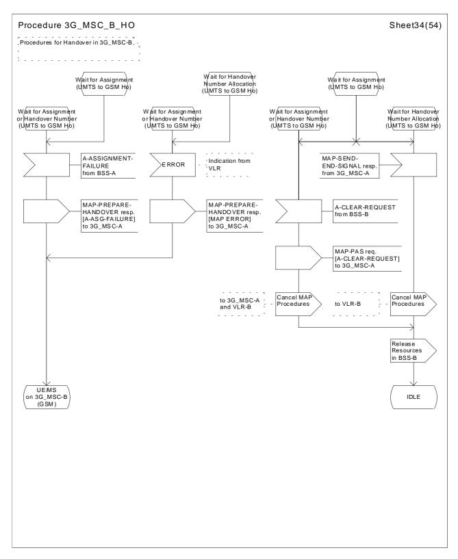
Figure 44 (sheet 34 of 54): Handover control procedure in 3G\_MSC-B
