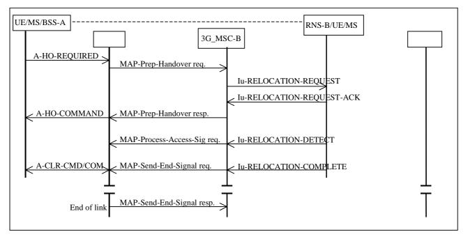
Figure 25: Basic GSM to UMTS Handover Procedure without circuit connection
