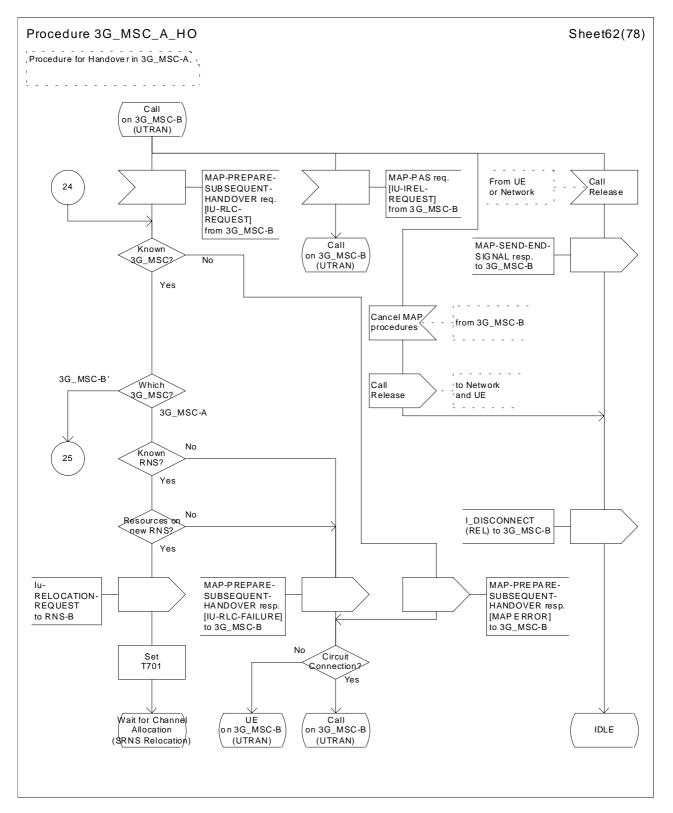
Figure 43 (sheet 62 of 78): Handover control procedure in 3G\_MSC-A
