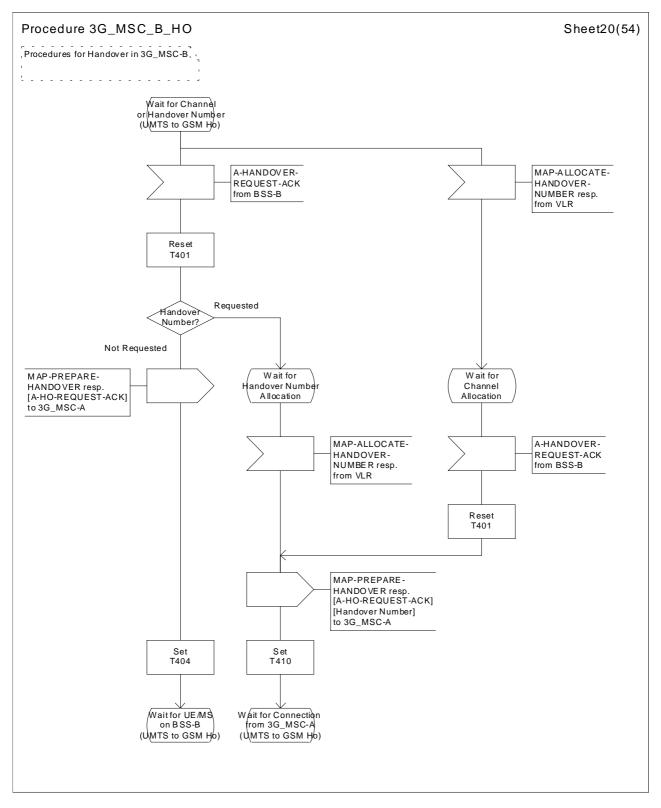
Figure 44 (sheet 20 of 54): Handover control procedure in 3G\_MSC-B
