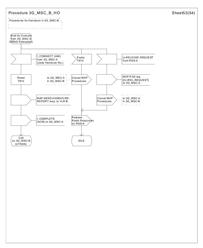
Figure 44 (sheet 53 of 54): Handover control procedure in 3G\_MSC-B
