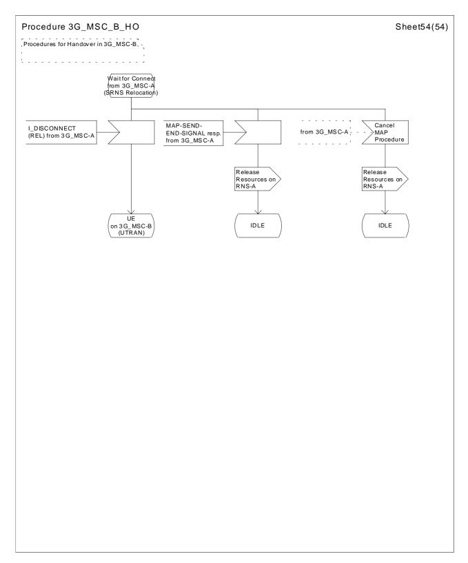
Figure 44 (sheet 54 of 54): Handover control procedure in 3G\_MSC-B
