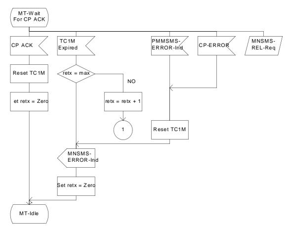
Note: The MNSMS-REL-Req is delayed until the next state
