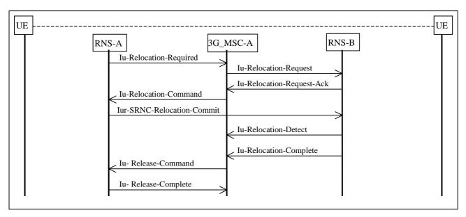
Figure 10 Basic intra-3G\_MSC SRNS Relocation Procedure
