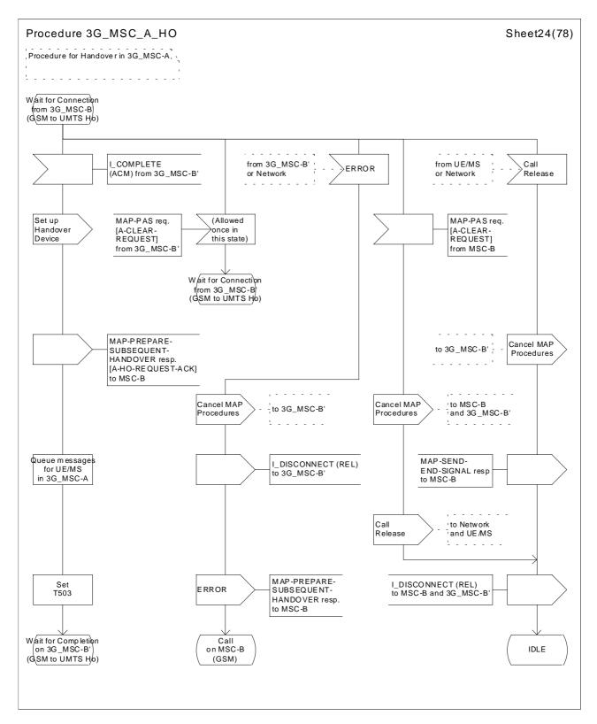
Figure 43 (sheet 24 of 78): Handover control procedure in 3G\_MSC-A
