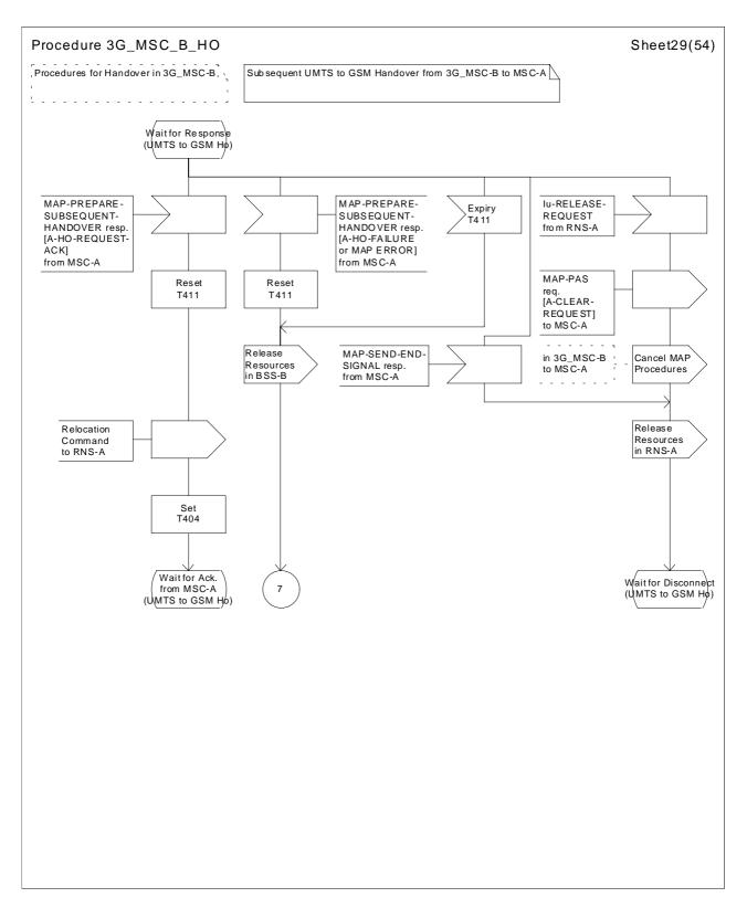
Figure 44 (sheet 29 of 54): Handover control procedure in 3G\_MSC-B
