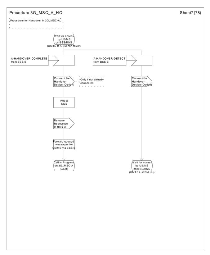
Figure 43 (sheet 7 of 78): Handover control procedure in 3G\_MSC-A
