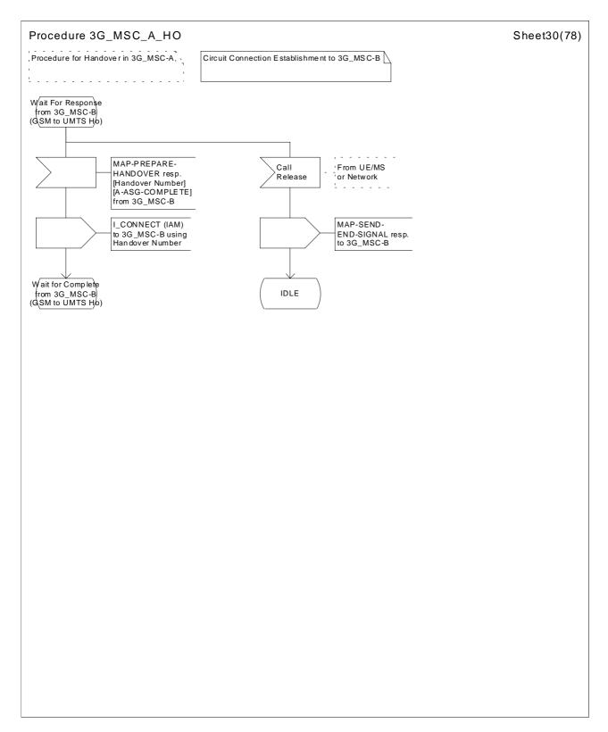
Figure 43 (sheet 30 of 78): Handover control procedure in 3G\_MSC-A
