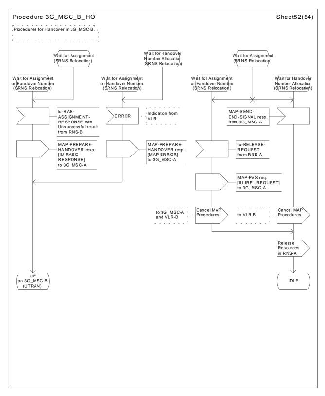
Figure 44 (sheet 52 of 54): Handover control procedure in 3G\_MSC-B
