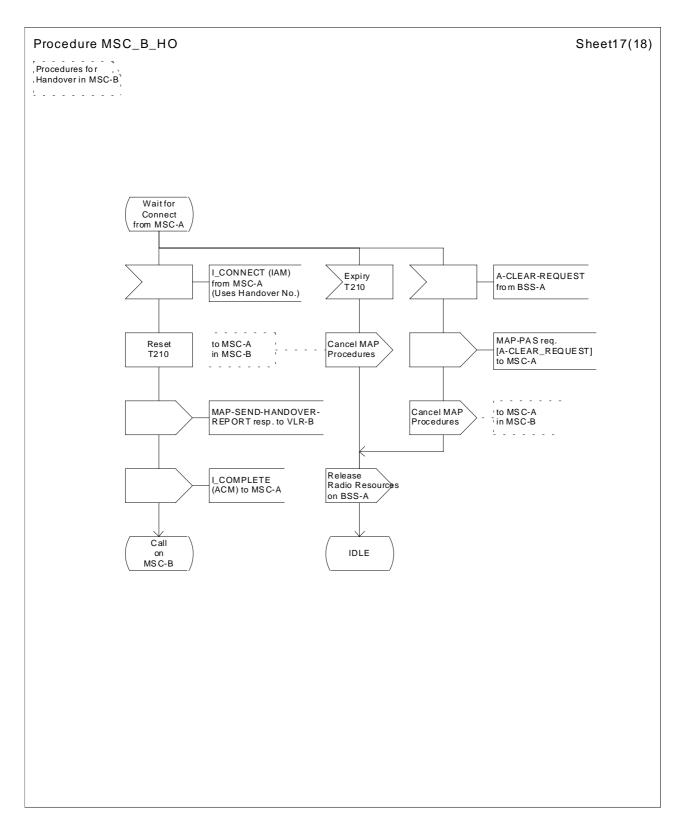
Figure 42 (Sheet 17 of 18): Handover control procedure in MSC-B
