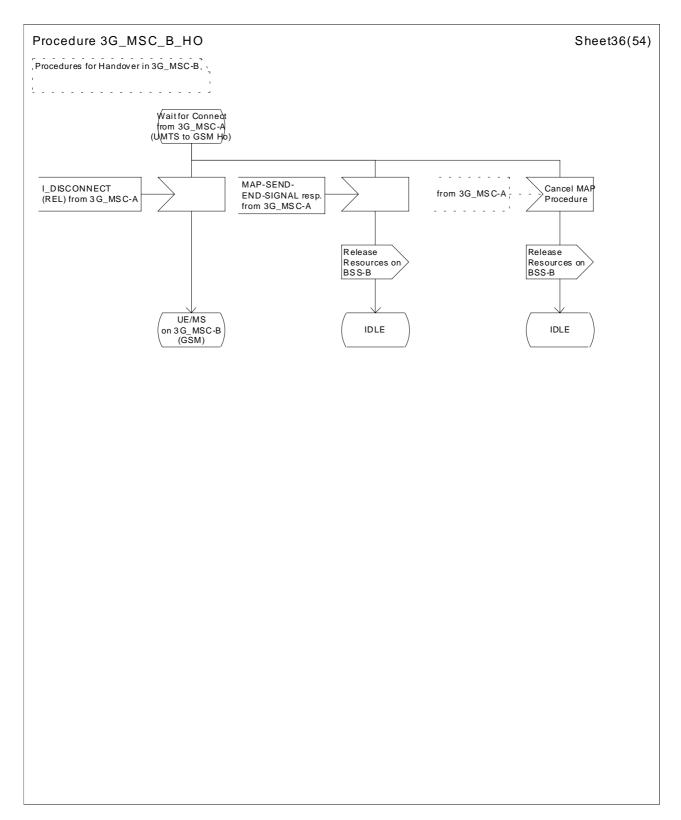
Figure 44 (sheet 36 of 54): Handover control procedure in 3G\_MSC-B
