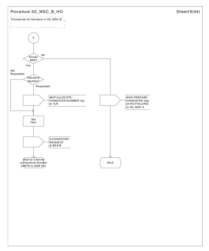
Figure 44 (sheet 19 of 54): Handover control procedure in 3G\_MSC-B
