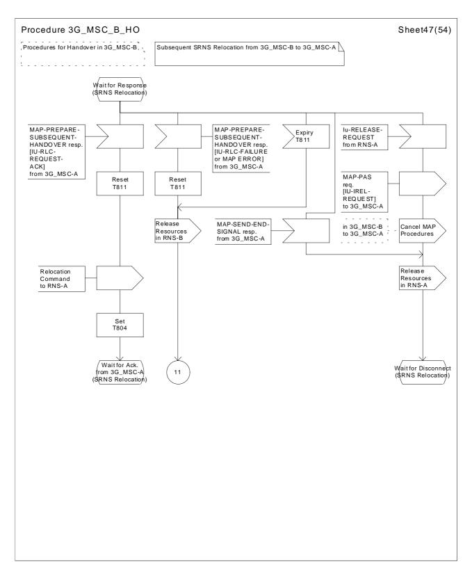
Figure 44 (sheet 47 of 54): Handover control procedure in 3G\_MSC-B
