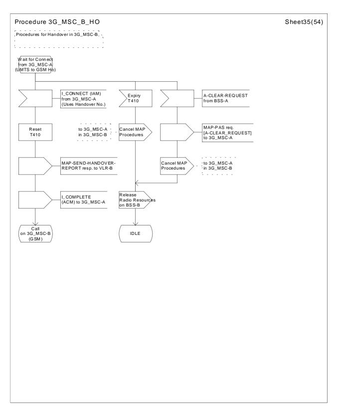
Figure 44 (sheet 35 of 54): Handover control procedure in 3G\_MSC-B
