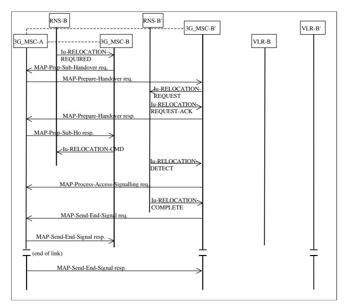
Figure 35: Subsequent relocation procedure ii) Successful SRNS relocation from 3G\_MSC-B to 3G\_MSC-B' not requiring a circuit connection
