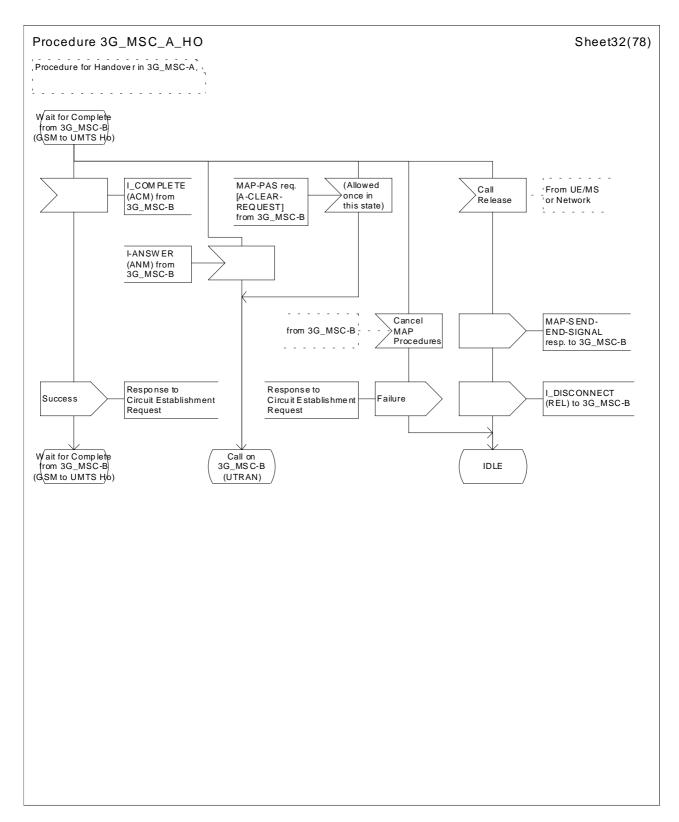
Figure 43 (sheet 32 of 78): Handover control procedure in 3G\_MSC-A
