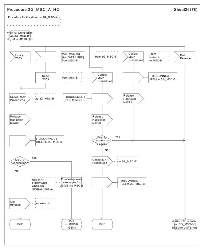
Figure 43 (sheet 26 of 78): Handover control procedure in 3G\_MSC-A
