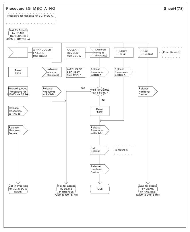
Figure 43 (sheet 4 of 78): Handover control procedure in 3G\_MSC-A
