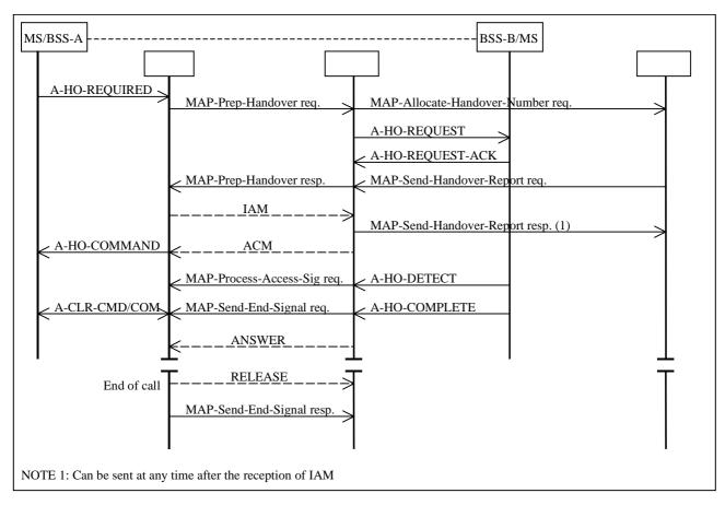
Figure 12: Basic Handover Procedure requiring a circuit connection
