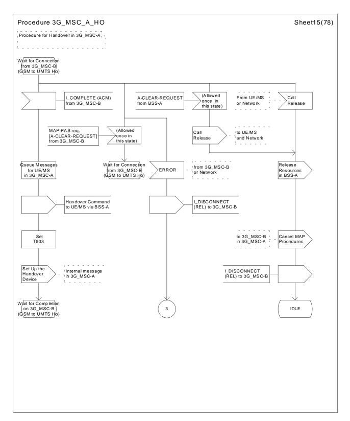
Figure 43 (sheet 15 of 78): Handover control procedure in 3G\_MSC-A
