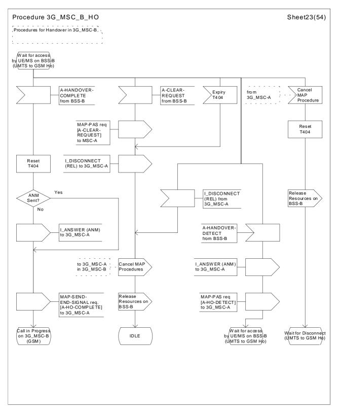
Figure 44 (sheet 23 of 54): Handover control procedure in 3G\_MSC-B
