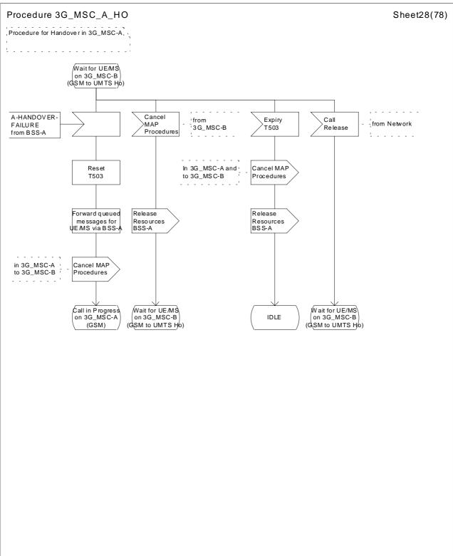
Figure 43 (sheet 28 of 78): Handover control procedure in 3G\_MSC-A
