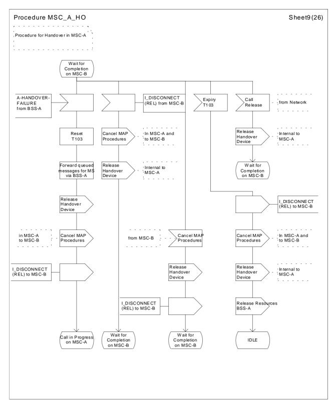
Figure 41 (Sheet 9 of 26): Handover control procedure in MSC-A
