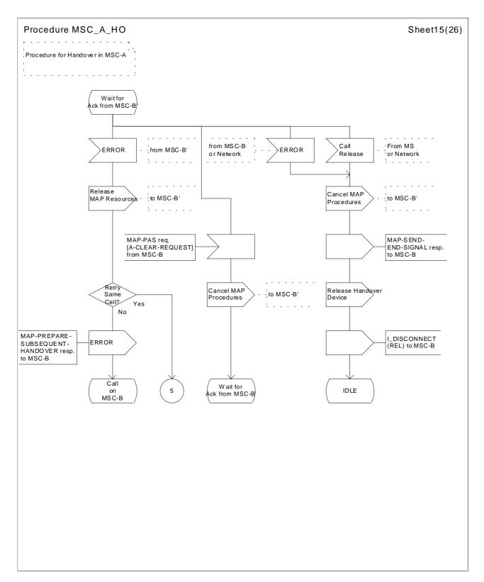
Figure 41 (Sheet 15 of 26): Handover control procedure in MSC-A
