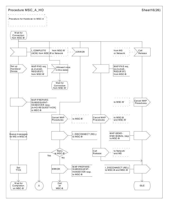
Figure 41 (Sheet 16 of 26): Handover control procedure in MSC-A
