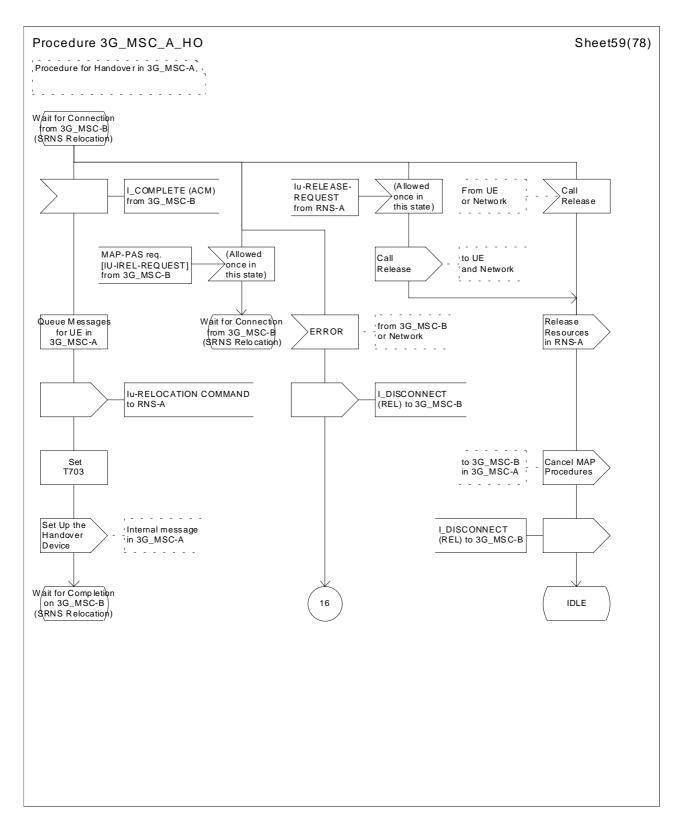
Figure 43 (sheet 59 of 78): Handover control procedure in 3G\_MSC-A
