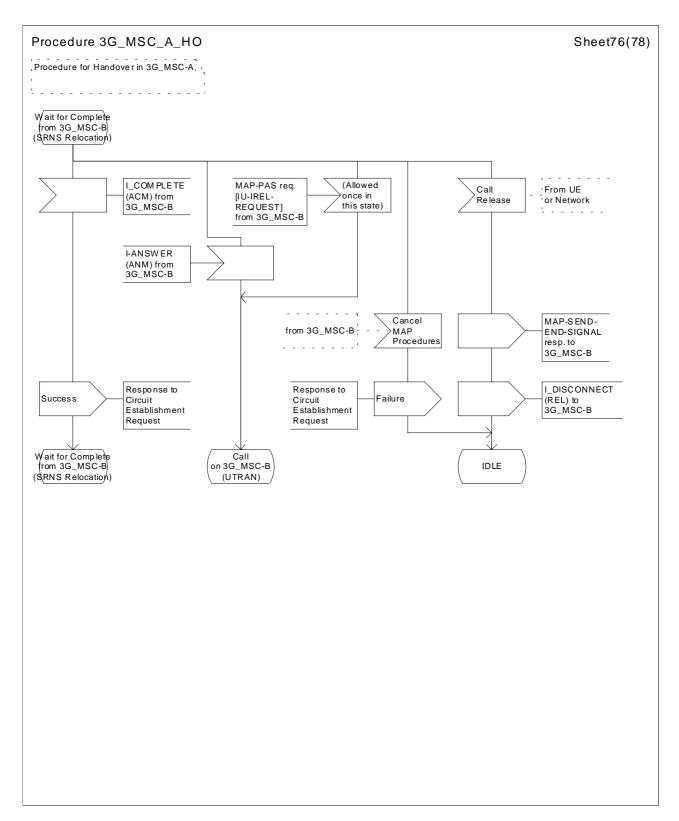
Figure 43 (sheet 76 of 78): Handover control procedure in 3G\_MSC-A
