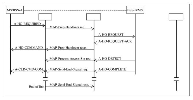
Figure 13: Basic Handover Procedure without circuit connection
