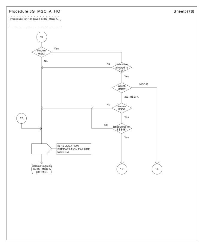
Figure 43 (sheet 5 of 78): Handover control procedure in 3G\_MSC-A
