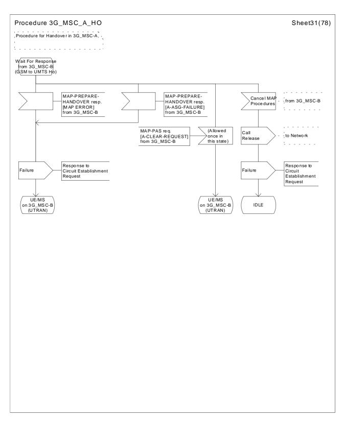
Figure 43 (sheet 31 of 78): Handover control procedure in 3G\_MSC-A
