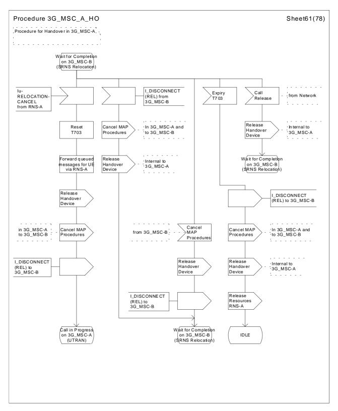
Figure 43 (sheet 61 of 78): Handover control procedure in 3G\_MSC-A
