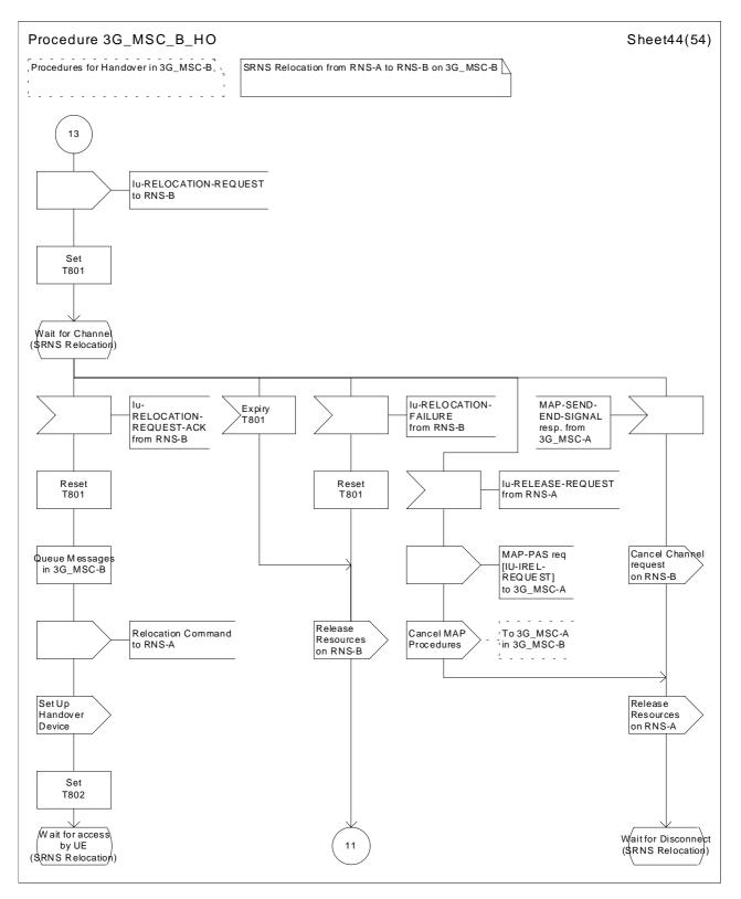
Figure 44 (sheet 44 of 54): Handover control procedure in 3G\_MSC-B
