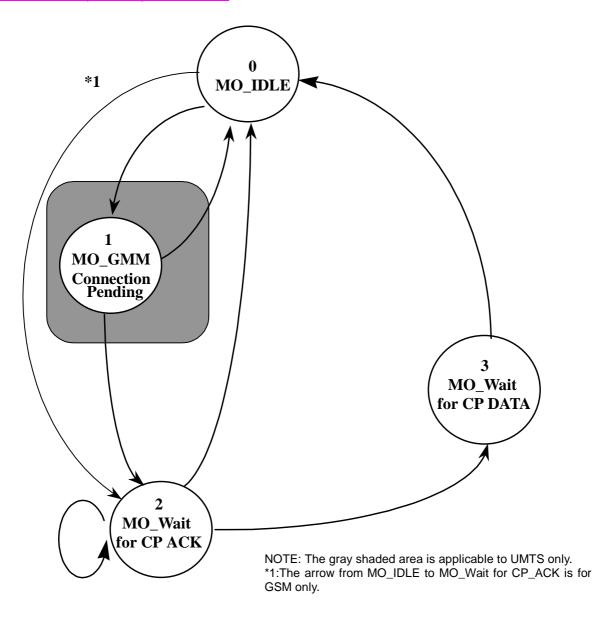
MO-SMC-GP entity on MS-side for GPRS State transition diagram
