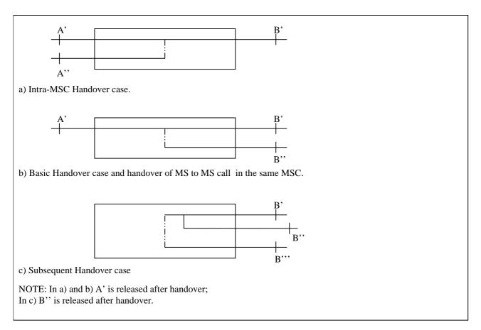
Figure 2: Connections in the handover device (Unit 5)
