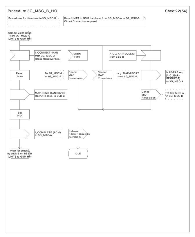
Figure 44 (sheet 22 of 54): Handover control procedure in 3G\_MSC-B
