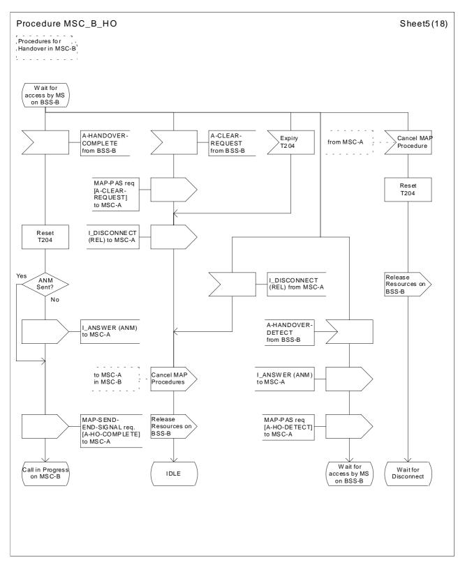
Figure 42 (Sheet 5 of 18): Handover control procedure in MSC-B
