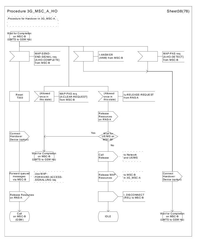
Figure 43 (sheet 38 of 78): Handover control procedure in 3G\_MSC-A
