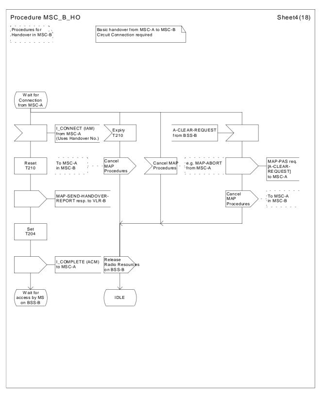
Figure 42 (Sheet 4 of 18): Handover control procedure in MSC-B
