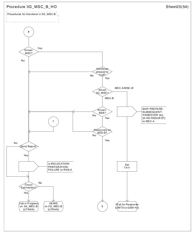
Figure 44 (sheet 25 of 54): Handover control procedure in 3G\_MSC-B
