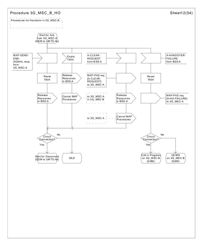
Figure 44 (sheet 12 of 54): Handover control procedure in 3G\_MSC-B
