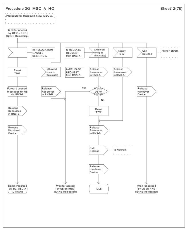
Figure 43 (sheet 12 of 78): Handover control procedure in 3G\_MSC-A
