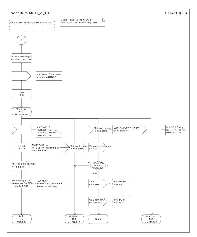
Figure 41 (Sheet 19 of 26): Handover control procedure in MSC-A
