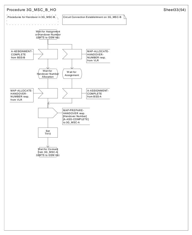
Figure 44 (sheet 33 of 54): Handover control procedure in 3G\_MSC-B
