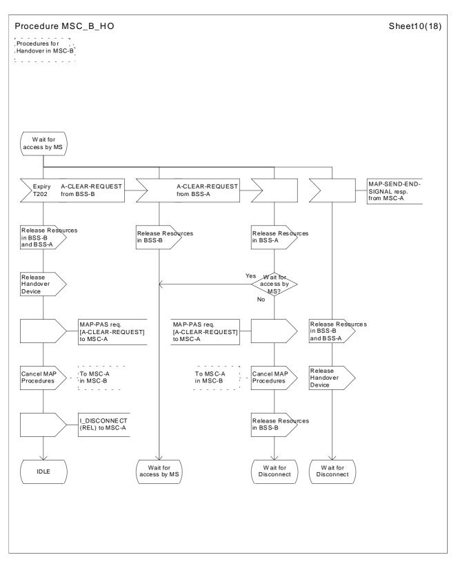
Figure 42 (Sheet 10 of 18): Handover control procedure in MSC-B
