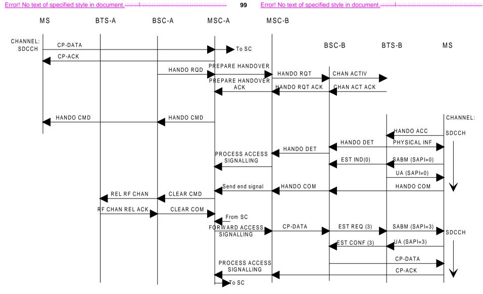
Figure F6/3GPP TS 24.011: Inter/MSC handover during Short Message transfer on SDCCH
