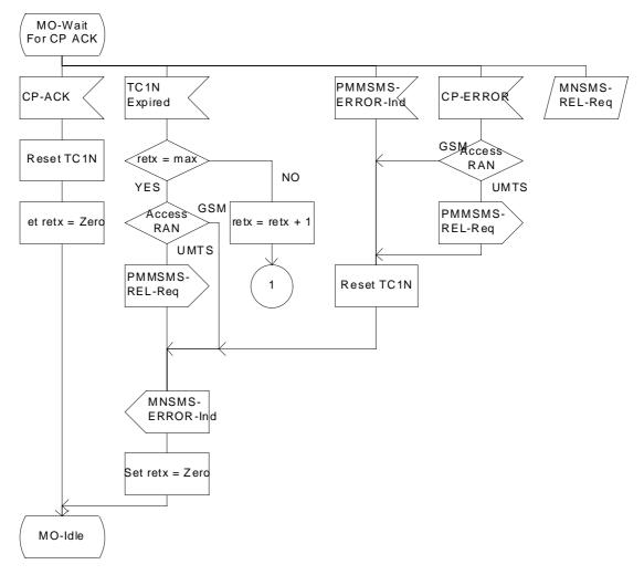
Note: The MNSMS-REL-Req is delayed until next state
