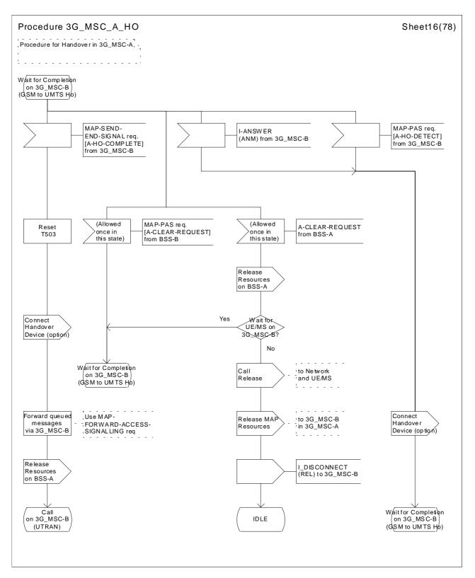
Figure 43 (sheet 16 of 78): Handover control procedure in 3G\_MSC-A
