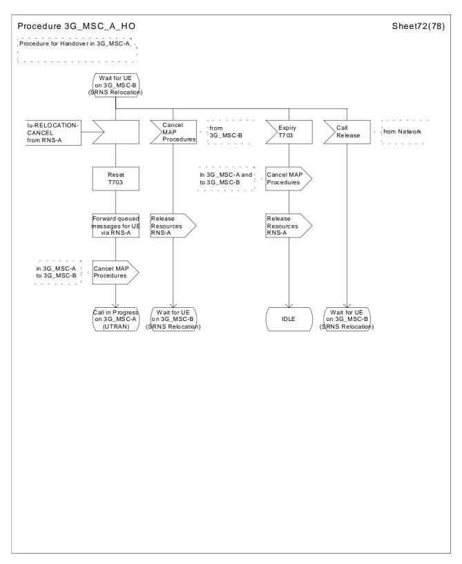
Figure 43 (sheet 72 of 78): Handover control procedure in 3G\_MSC-A
