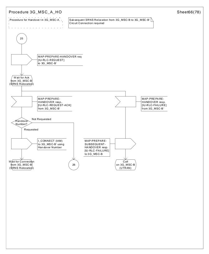
Figure 43 (sheet 66 of 78): Handover control procedure in 3G\_MSC-A
