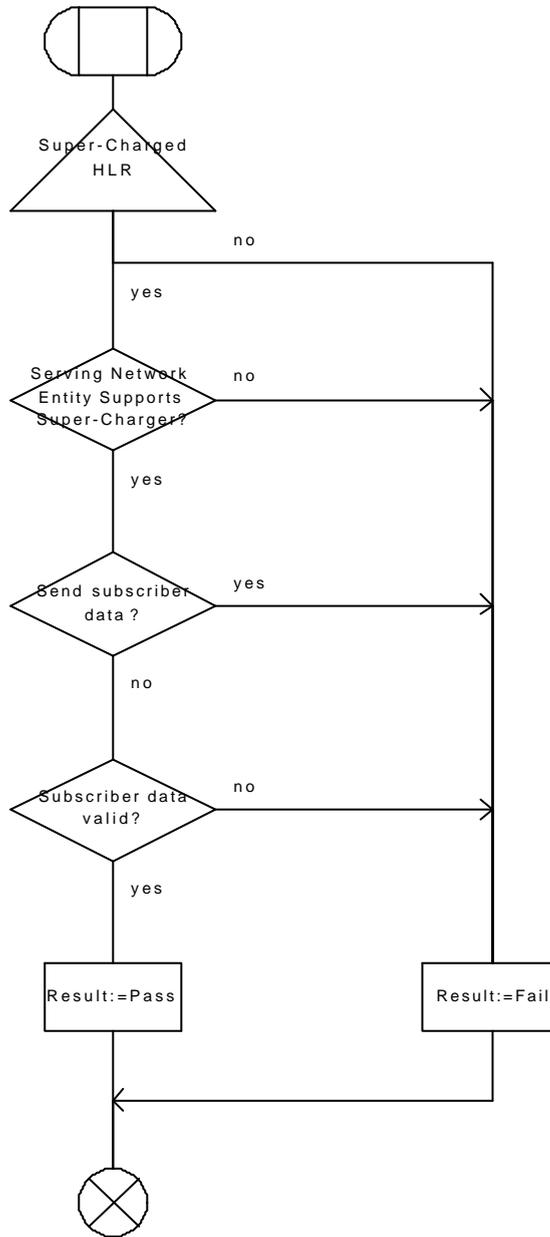
Figure 6: Procedure Super\_Charger\_Location\_Updating\_HLR
