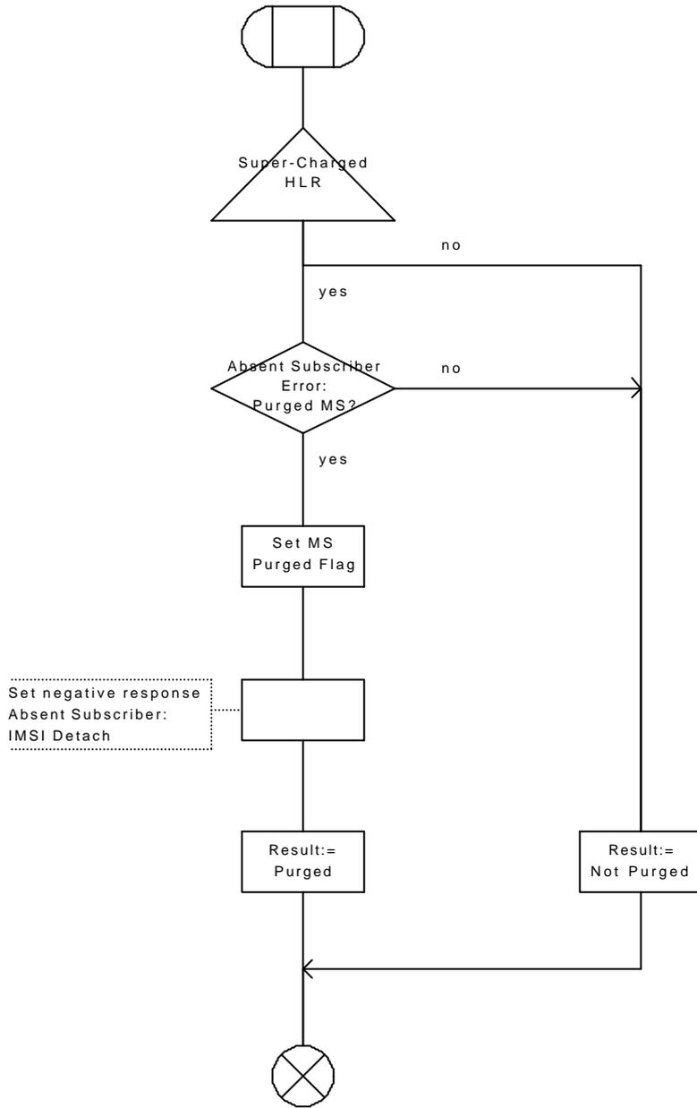
Figure 10: Procedure Super\_Charged\_SRI\_Error\_HLR
