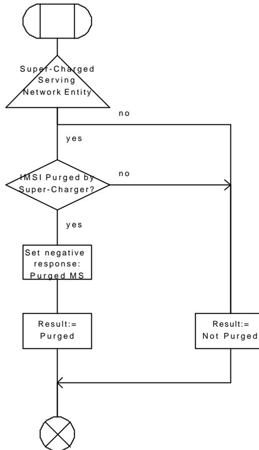
Figure 9: Procedure Check\_Reason\_In\_Serving\_Network\_Entity
