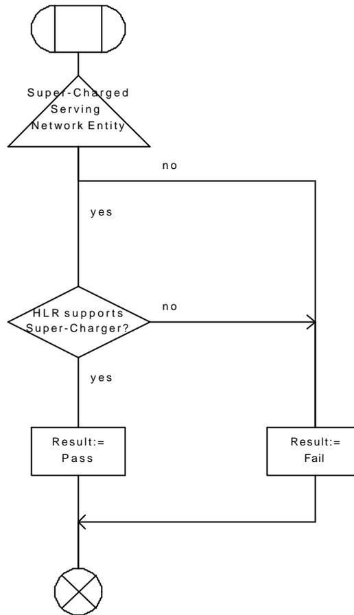
**Figure 8: Procedure Purge\_MS\_In\_Serving\_Network\_Entity**
