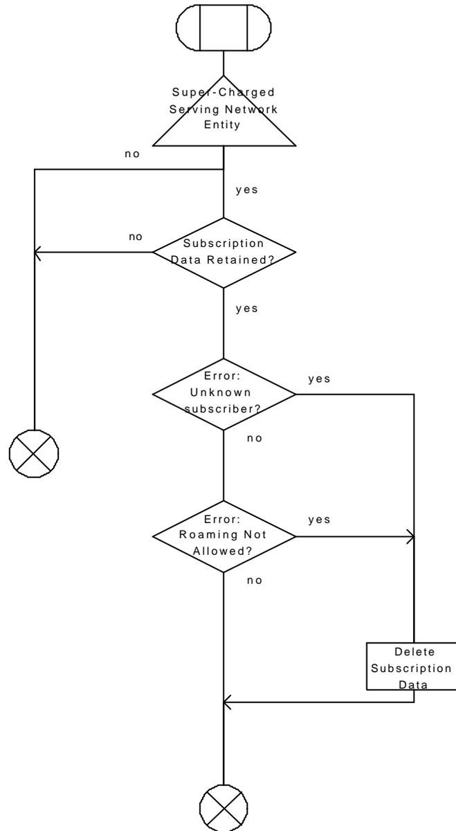
Figure 5: Procedure Check\_User\_Error\_In\_Serving\_Network\_Entity
