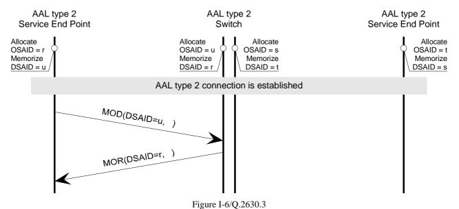
Example of a message sequence for an unsuccessful resource modification of an established AAL type 2 connection
