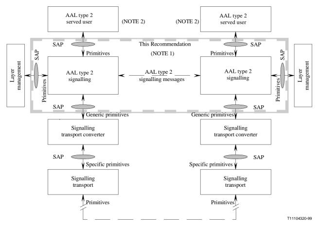
NOTE 1 - The entities and Service Access Points (SAP) bounded by the gray broken line indicate the extent of the definitions specified in this Recommendation.
