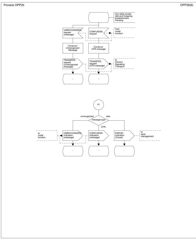
Figure 8-2/Q.2630.3 (Part 6 of 6) SDL Diagram for the Outgoing Protocol Procedure
