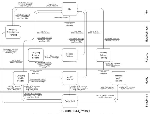
State transition diagram for the outgoing protocol procedure
