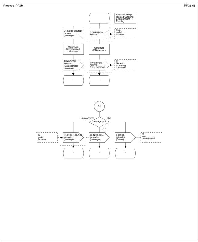
Figure 8-4/Q.2630.3 (Part 6 of 6) SDL Diagram for the Incoming Protocol Procedure
