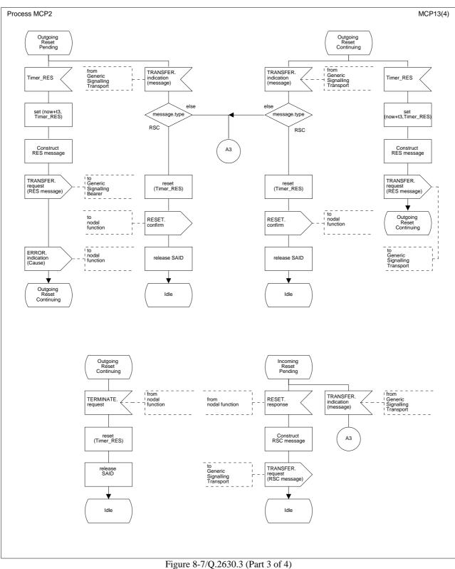
SDL diagram for the maintenance control procedure
