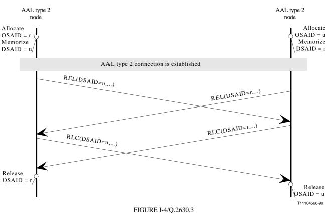
Example of a message sequence for a release collision on an AAL type 2 connection
