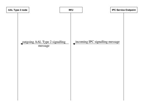
Figure 2/Q.2632.1 – IPC to AAL type 2 signalling interworking
