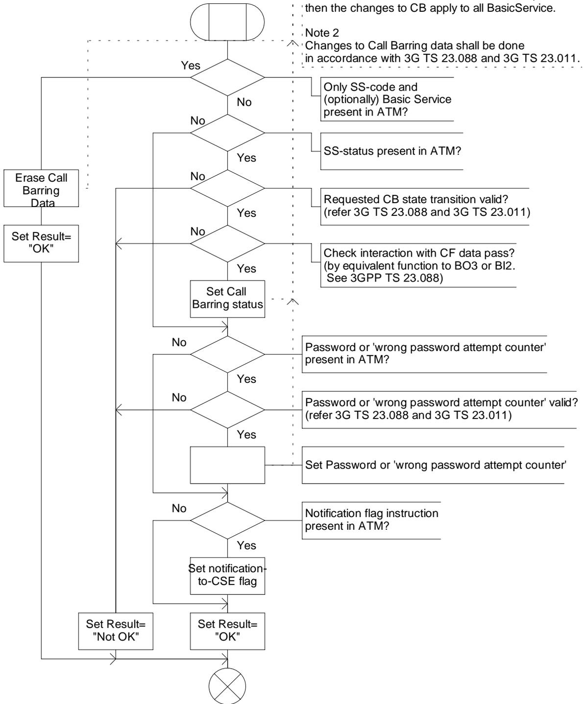
Figure 10.7: Procedure ATM\_Modify\_CB\_Data (sheet 1)
