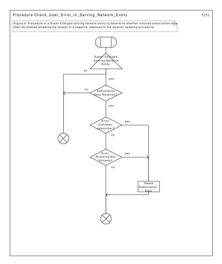
Figure 5: Procedure Check\_User\_Error\_In\_Serving\_Network\_Entity
