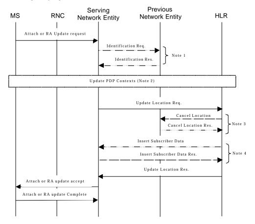
Note 1: This procedure is optionally performed as part of the Attach procedures, see TS 23.060.
