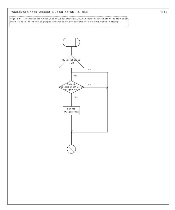
Figure 11: Procedure Check\_Absent\_SubscriberSM\_In\_HLR
