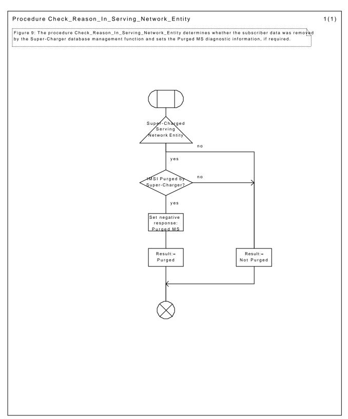
Figure 9: Procedure Check\_Reason\_In\_Serving\_Network\_Entity
