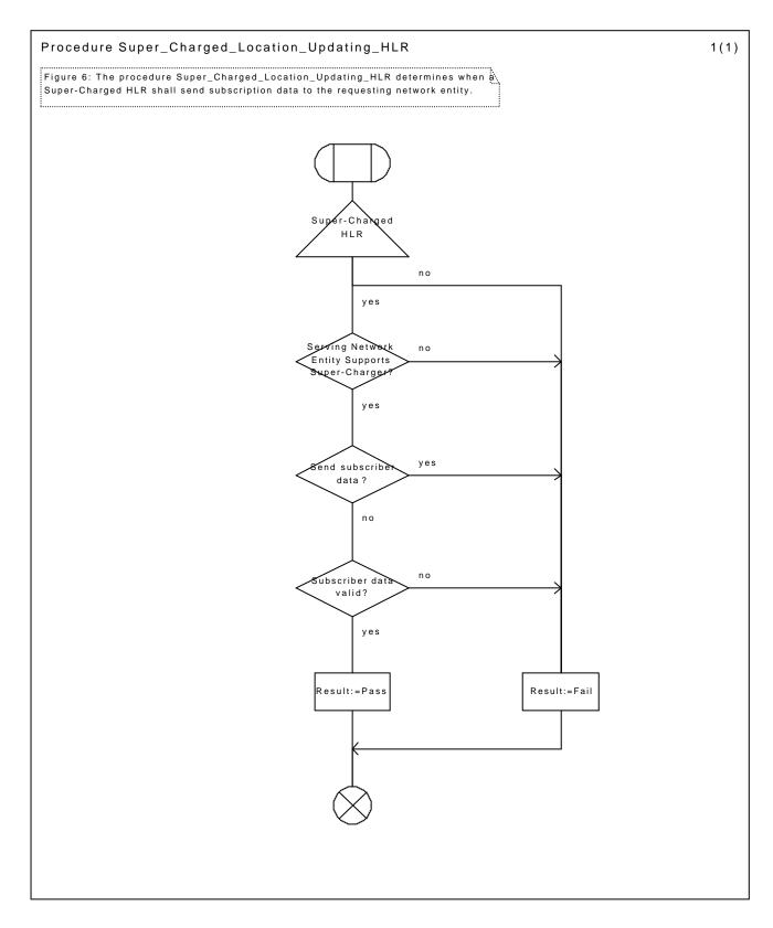
Figure 6: Procedure Super\_Charger\_Location\_Updating\_HLR
