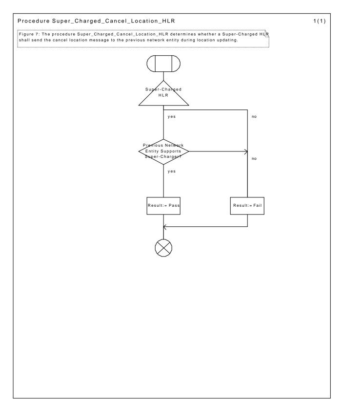
Figure 7: Procedure Super\_Charged\_Cancel\_Location\_HLR
