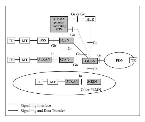
Figure 1: GPRS Logical Architecture with interface name denotations
