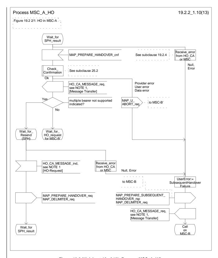
Figure 19.2.2/1 (sheet 10 of 13): Process MSC\_A\_HO
