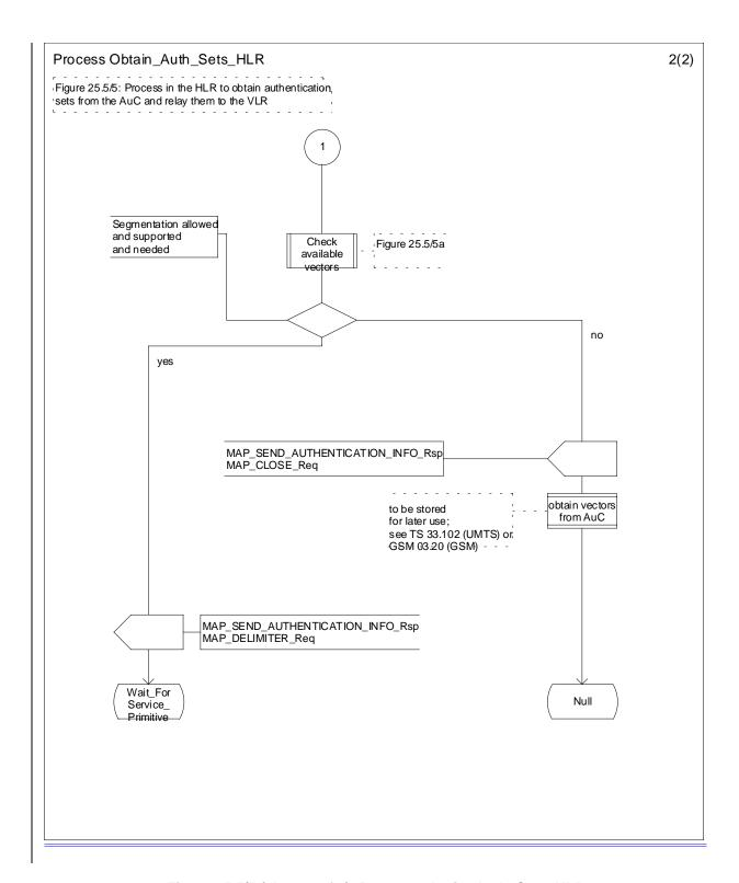
Figure 25.5/5 (sheet 2 of 2): Process Obtain\_Auth\_Sets\_HLR
