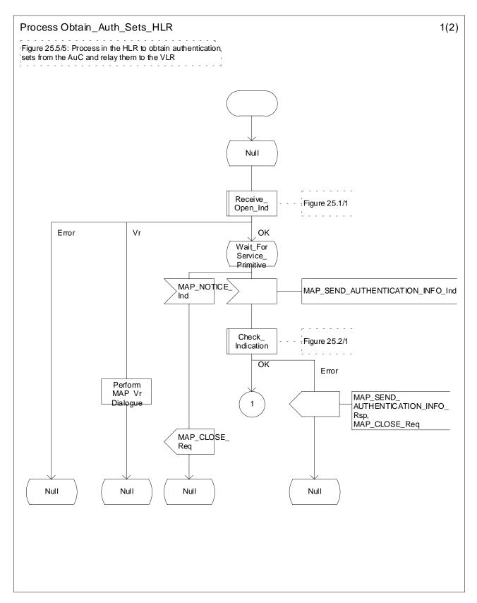
Figure 25.5/5 (sheet 1 of 2): Process Obtain\_Auth\_Sets\_HLR
