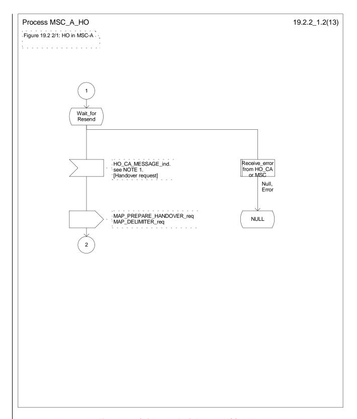
Figure 19.2.2/1 (sheet 2 of 13): Process MSC\_A\_HO
