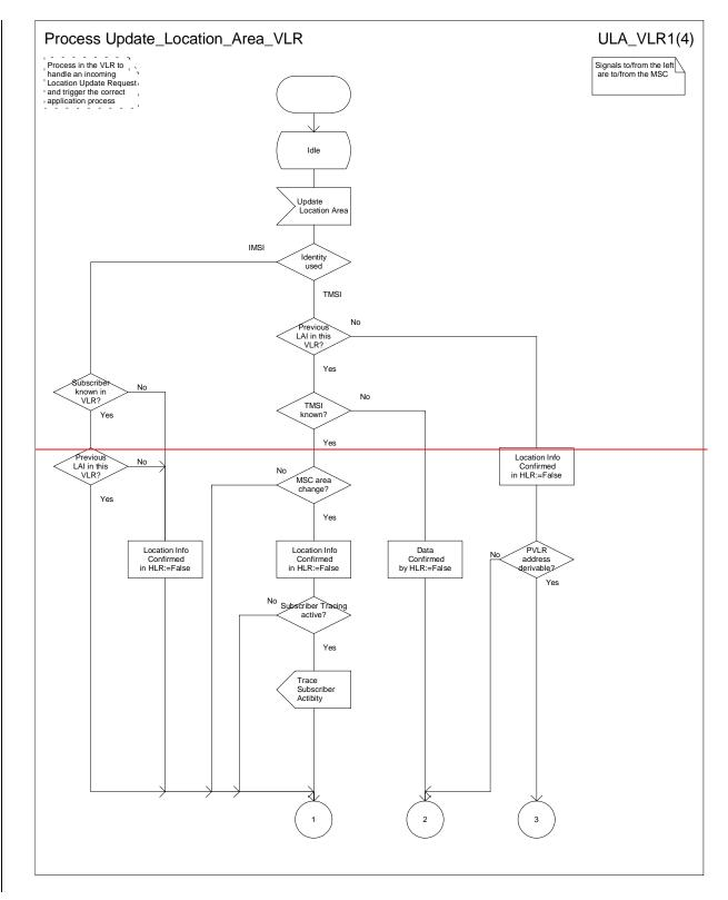
Figure 4.1.2.1 (sheet 1 of 4): Process Update\_Location\_Area\_VLR
