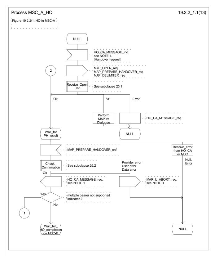
Figure 19.2.2/1 (sheet 1 of 13): Process MSC\_A\_HO
