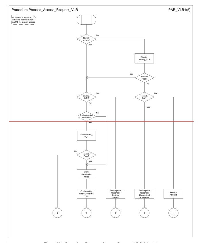
Figure 20a: Procedure Process\_Access\_Request\_VLR (sheet 1)
