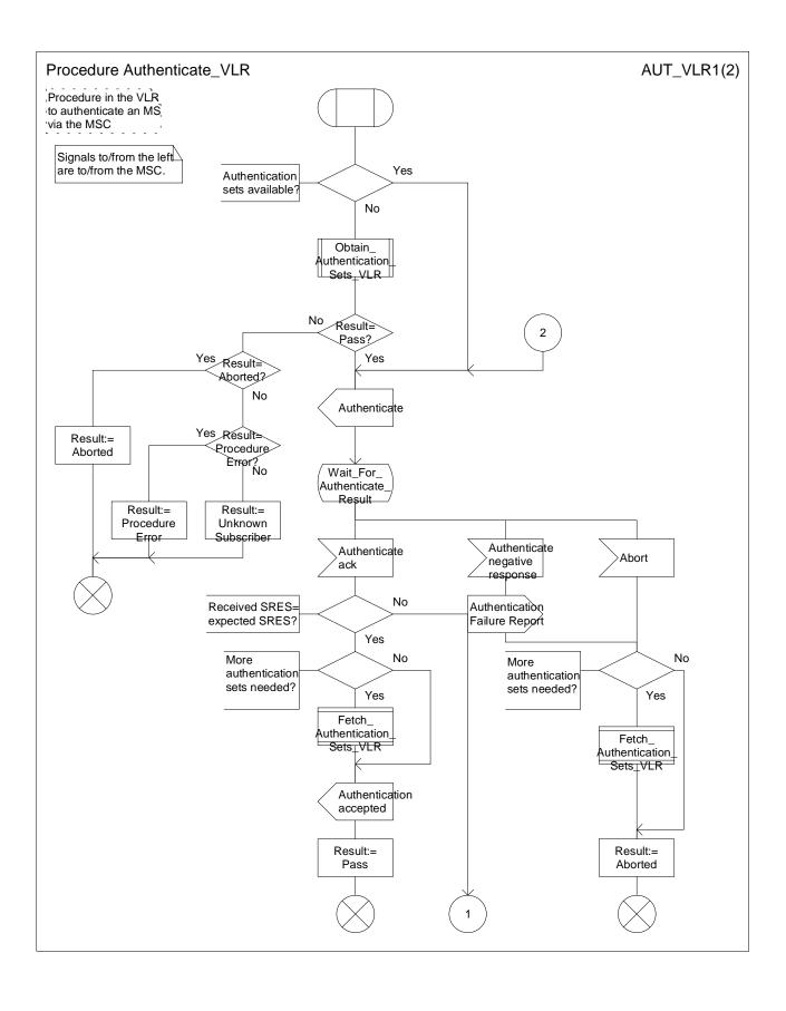
Figure 1a: Procedure Authenticate\_VLR (sheet 1)
