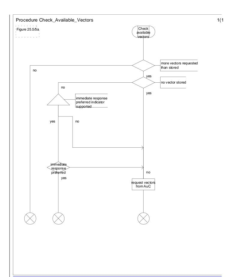
Figure 25.5/5a: Procedure Check\_Available\_Vectors
