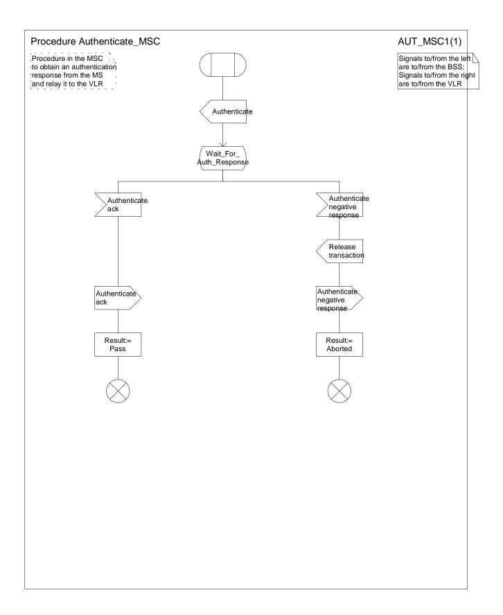
Figure 4.1.1.2 (sheet 1 of 1): Procedure Authenticate\_MSC
