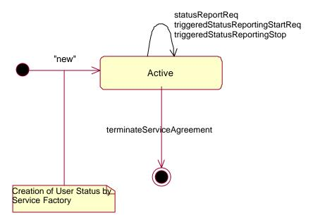
Figure 7-16: State Transition Diagram for User Status.
