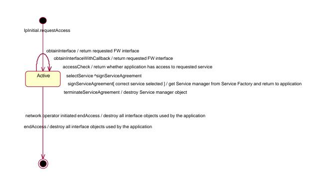
Figure 7-2: State Transition Diagram for Access
