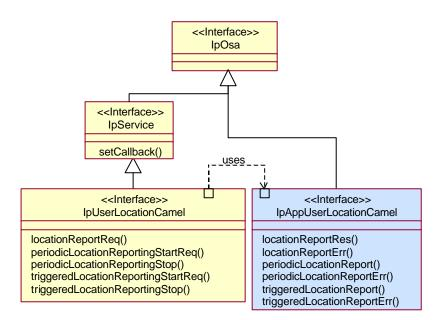
Figure 6-12: Network User Location class diagram.
