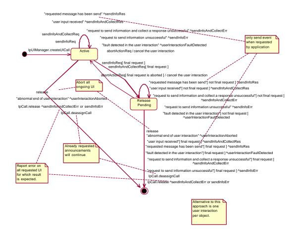
Figure 7-14: State Transition Diagram for UICall
