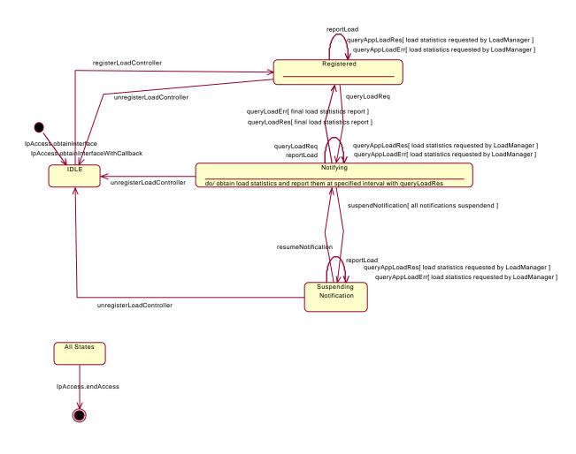
Figure 7-4: State Transition Diagram for LoadManager
