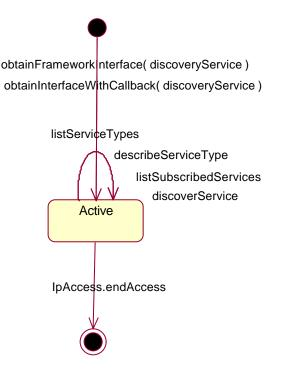
Figure 7-3: State Transition Diagram for Service Discovery
