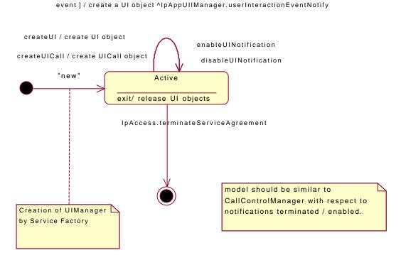
Figure 7-12: State Transition Diagram for the UIManager
