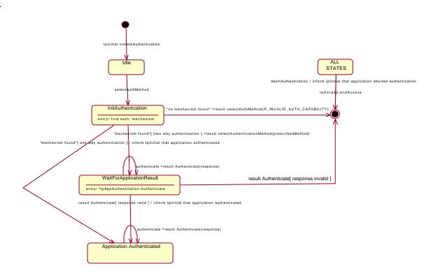
Figure 7-1: State Transition Diagram for Authentication
