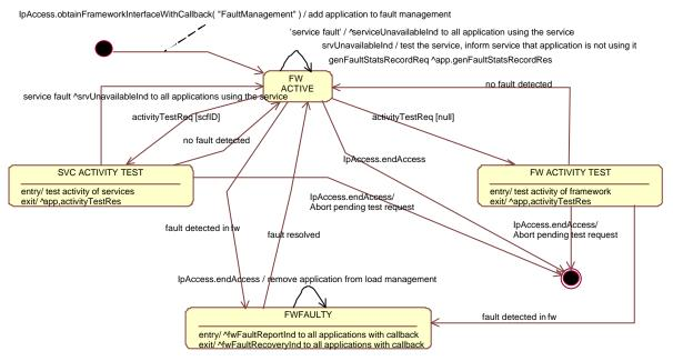
Figure 7-6: State Transition Diagram for Fault Manager
