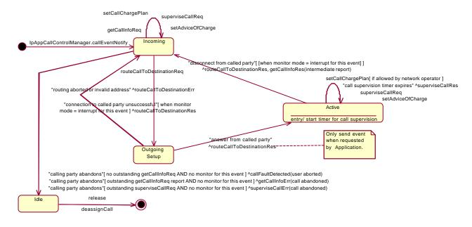
Figure 7-10: State Transition Diagram for Call, part 1
