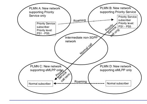
Figure B-9. Priority Service call terminating to an eMLPP network
