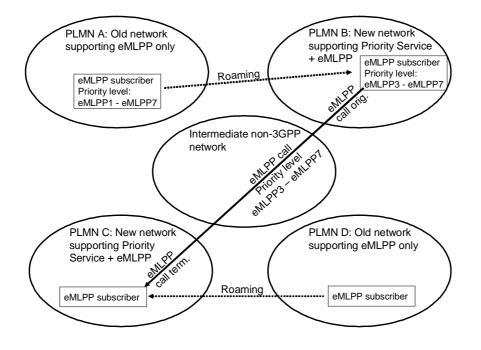
Figure <u>B-</u>6 - eMLPP call to eMLPP subscriber in Priority Service + eMLPP network
