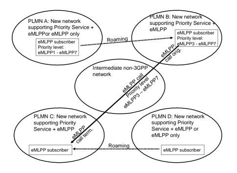
Figure <u>B-</u>2. eMLPP call to eMLPP subscriber in Priority Service + eMLPP network
