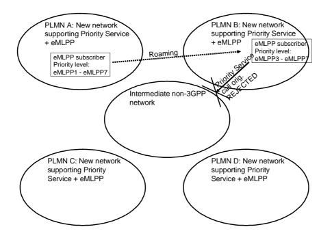
Figure  $\underline{B}$ -8 - An eMLPP subscriber roams to a Priority Service + eMLPP network and initiates a call with the Priority Service service code
