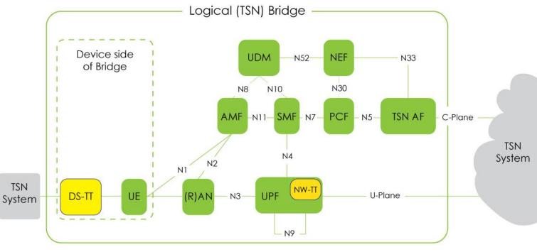
System architecture view with 5GS appearing as a Time-Sensitive Networking bridge
