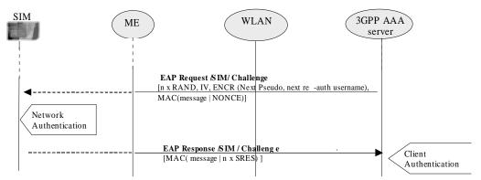
Fig 3: Network authentication example in EAP-SIM with EAP support for smartcards
