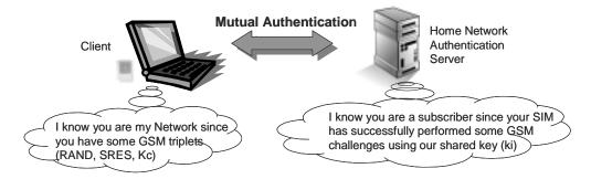
An attacker that knows some subscriber's GSM triplets can simulate a fake network and mount a man-in-the-middle attack extremely compromising the user security.
