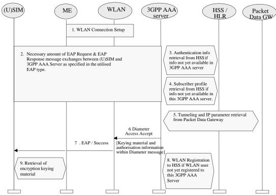
Figure: Authentication procedure based on EAP support in smartcards
