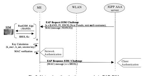
Fig 2: Network authentication example in EAP-SIM
