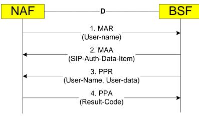
Figure 5: Two phases Cx based Bootstrapping Procedure in C interface – Alternative 1
