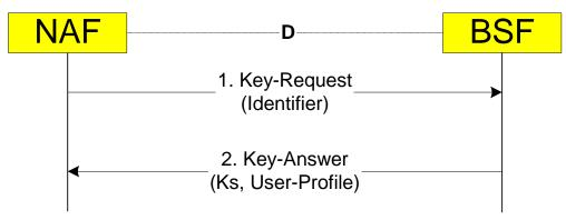
Figure 4: The Bootstrapping Procedure in C interface
