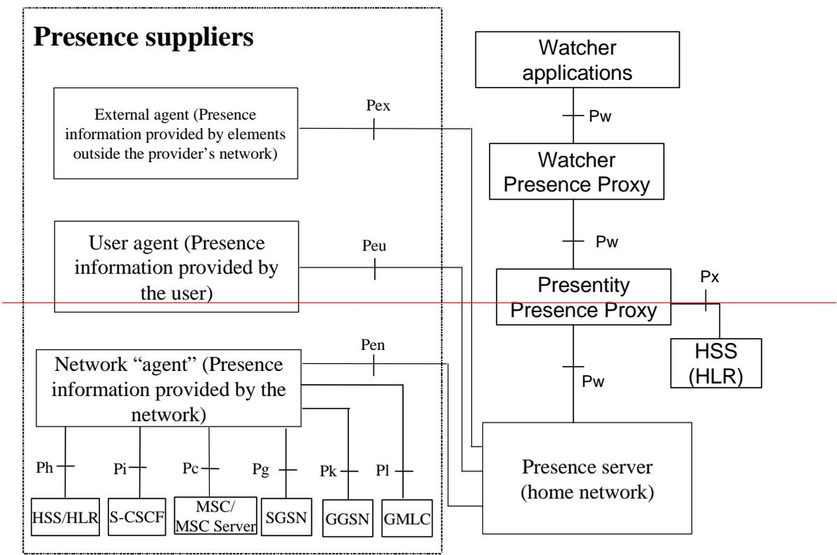
Interfaces Ph, Pi, Pc, Pg, Pk and Pl are based on existing R5 procedures e.g. CAMEL, MAP, CAP, RADIUS, ISC, Cx, Sh.
