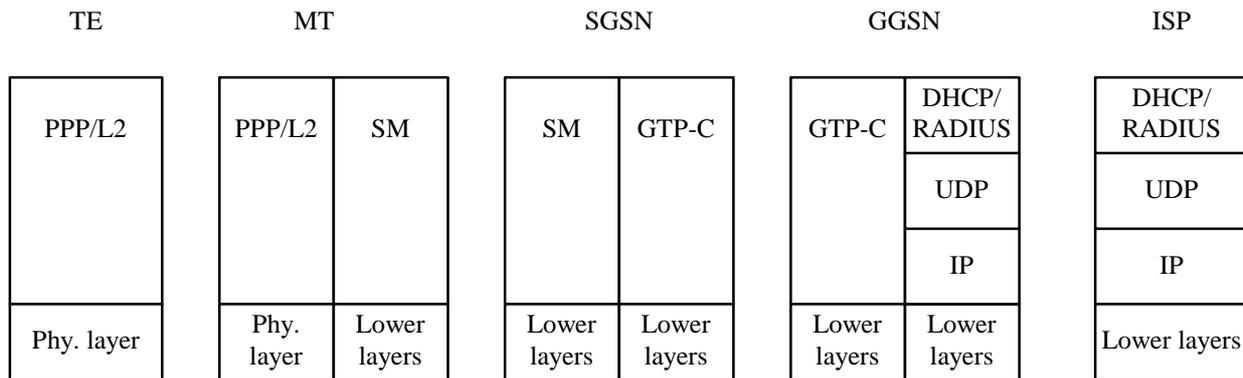
Figure 11a: Signalling plane of non transparent case
