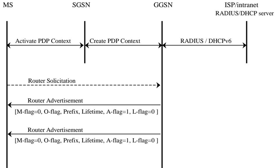
**Figure 11bbd: IPv6 Stateless Address Autoconfiguration**
