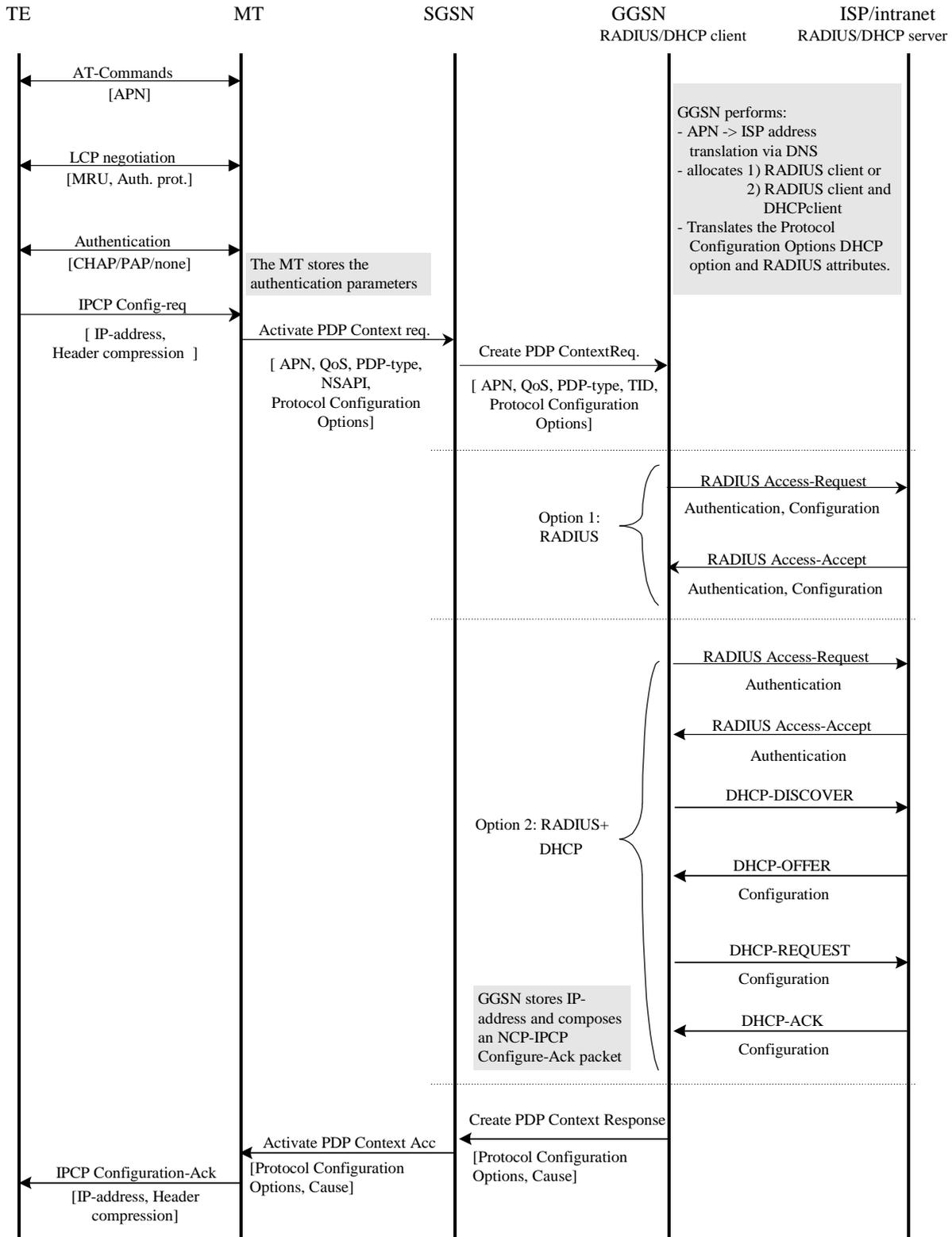
Figure 11b: PDP Context Activation for the IPv4 Non-transparent IP case
