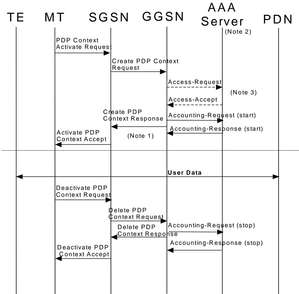
NOTE 1: If some external applications require RADIUS Accounting request (Start) information before they can process user packets, then the selected APN (GGSN) may be configured in such a way that the GGSN drops user data until the Accounting Response (START) is received from the AAA server. Both Authentication and Accounting servers may be optional and separately configured for each APN.
