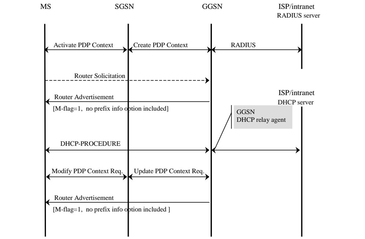
**Figure 11bc: IPv6 Stateful Address Autoconfiguration**
