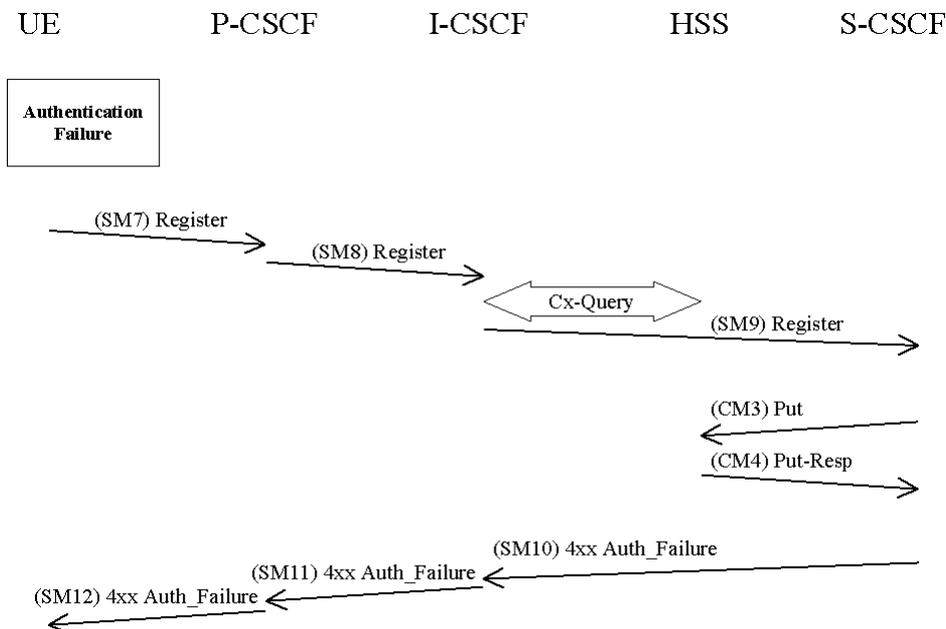
The UE shall send a Register message towards the HN including an indication of the cause of failure in SM7. The P-CSCF and the I-CSCF forward this message to the S-CSCF.
