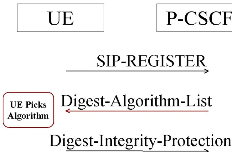
This security mode set-up looks different to the current requirements defined in clause 7 where the P-CSCF chooses the algorithm. A proposed mechanism for bidding down protection is to utilise a nonce, which will have a meaning for the client. The nonce-value in this case is not longer only a random number it will include the integrity algorithm and quality of protection along with the traditional nonce value. The nonce in this case could look like:
