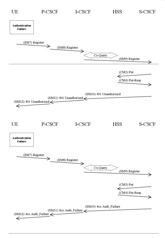
The UE shall send a Register message towards the HN including an indication of the cause of failure in SM7. The P-CSCF and the I-CSCF forward this message to the S-CSCF.
