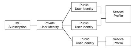
According to the SA1 requirement this is the scenario that should be supported by the IMS in Release 5. All public user identities that are associated with the same profile should have the same set of services. Public user identities that are associated with a different profile could have a different set of services.]
