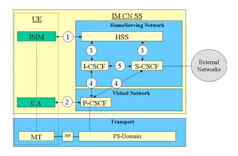
Figure 1. The This is the security IMS security architecture for the IM CN Subsystem.
