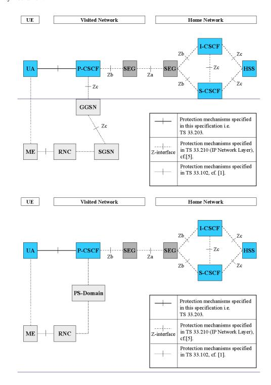
Figure 2. This figure gives an overview of the security architecture for <u>IM-CN-SSIMS</u> and the relation with Network Domain security, cf. [5].
