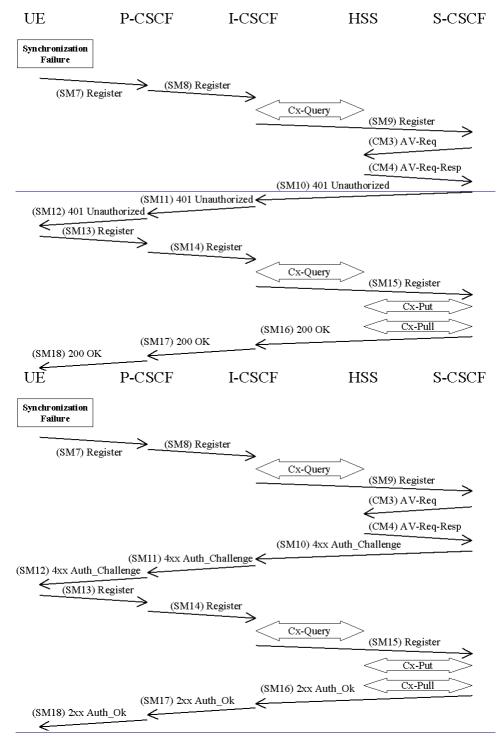
The flow equals the flow in 6.1.3.1 up to SM6. When the UE receives SM6 it detects that the SQN is out of range and sends a synchronization failure back to the S-CSCF in SM7.
