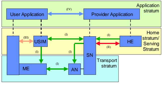
Figure 1 gives an overview of the complete 3G security architecture.
