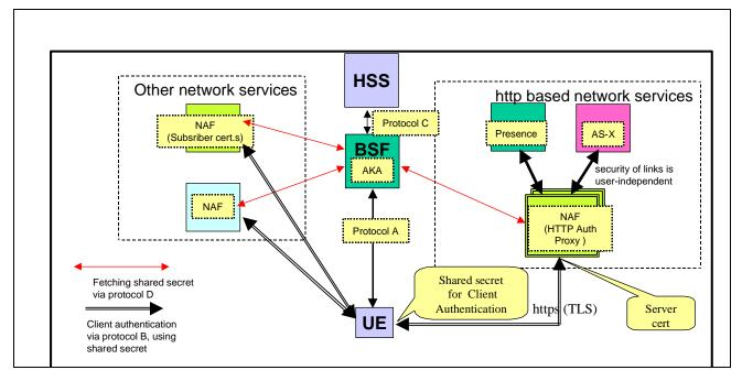
When the UE wants to access one of the application servers, which are attached to the AP, on the right hand side of the figure, then the sequence of events is as follows (overview):
