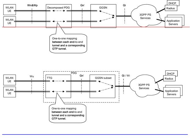
Figure F.2: Mapping between E2E tunnel and GTP tunnel
