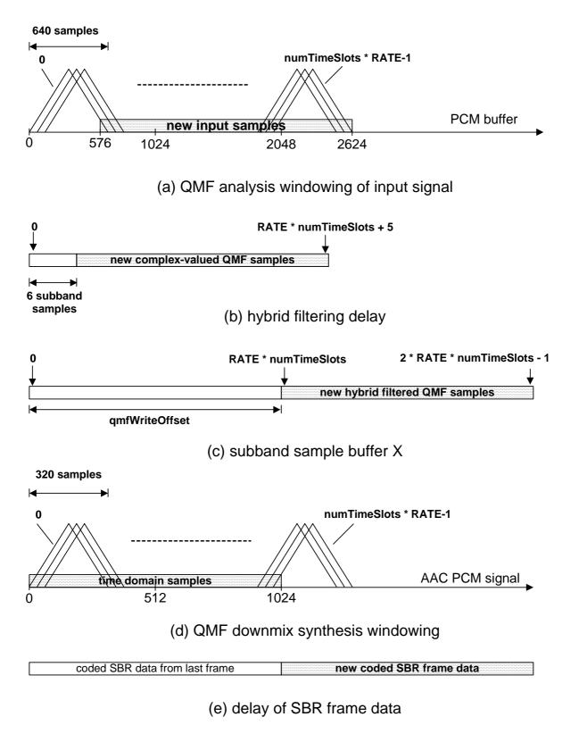
Figure 4 Enhanced aacPlus stereo synchronisation
