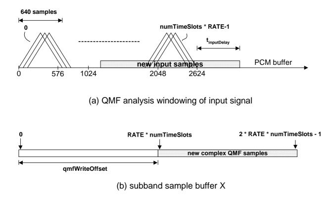
Figure 3 aacPlus encoder buffers and synchronisation
