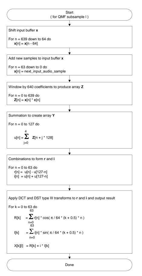
Figure 6 – Flowchart of encoder analysis QMF bank
