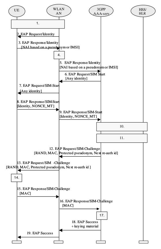
Figure 5: Authentication based on EAP SIM scheme
