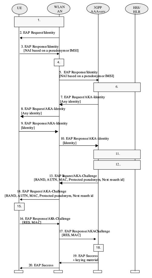
Figure 4: Authentication based on EAP AKA scheme
