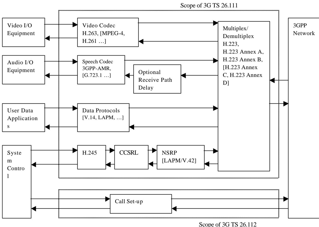
Figure 1 Scope of circuit switched multimedia 3GPP specification.
