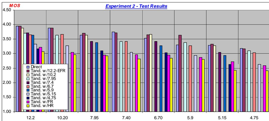
Figure 7.1: Experiment 2 Test Results (cross-codec tandeming)
