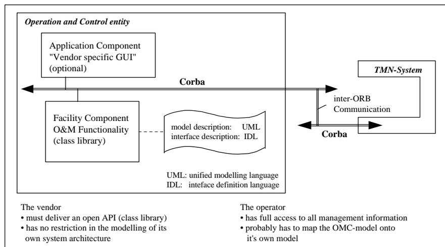
***Figure 1 Conceptual Architecture of an O&M-Transformer***
