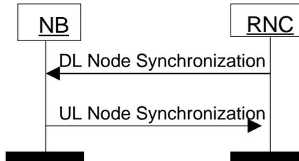
**Figure X. “Channel”DCH Node Synchronization procedure.**
