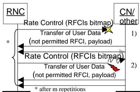
Figure x. Unsuccessful Transfers of rate control: 1) Frame loss 2) Corrupted Frame
