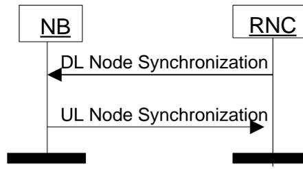
**Figure X. "Channel" Node Synchronization procedure.**
