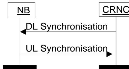
**Figure 6. FACH and PCH Synchronisation procedure.**
