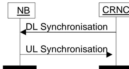
**Figure 7. DSCH Synchronisation procedure.**
