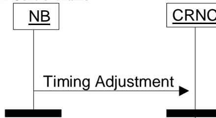
Figure 9. DSCH Timing Adjustment procedure.
