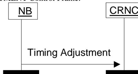
**Figure 8. FACH and PCH Timing Adjustment procedure.**
