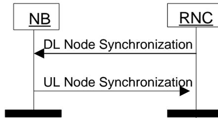
**Figure 5. Node Synchronisation procedure.**
