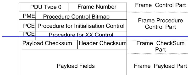
**Figure 4: lu UP PDU Type 0 Format**
