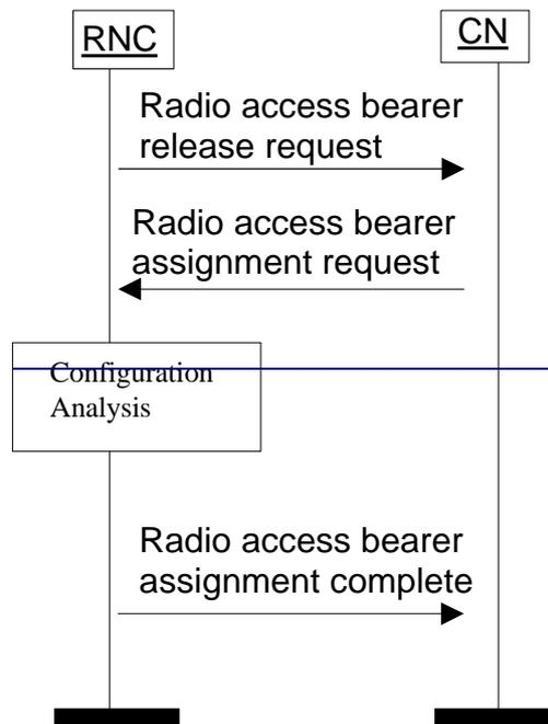
**Figure 8. Radio Access Bearer Assignment procedure, UTRAN generated release.**
