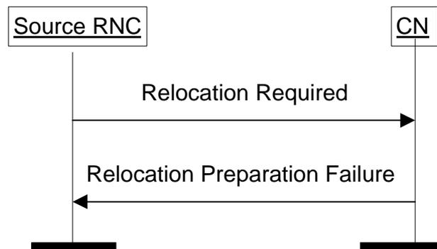
**Figure 2. Relocation preparation failure.**
