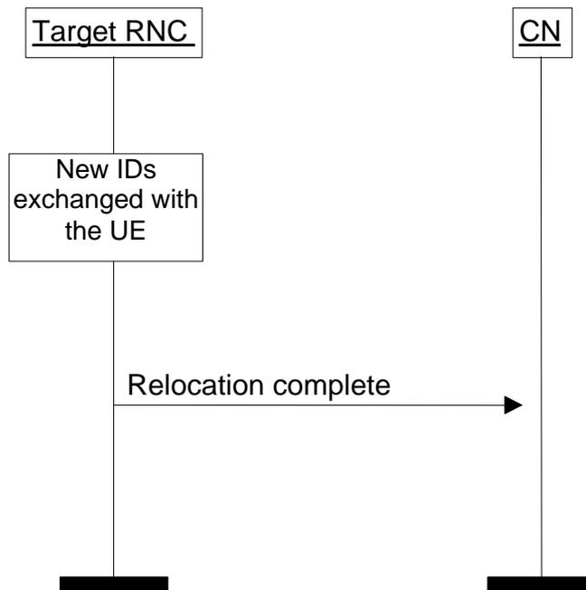
Figure 667. Relocation Complete procedure.
