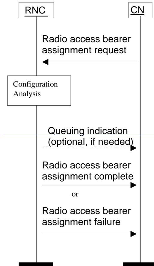
Figure 9. Radio Access Bearer Assignment procedure.
