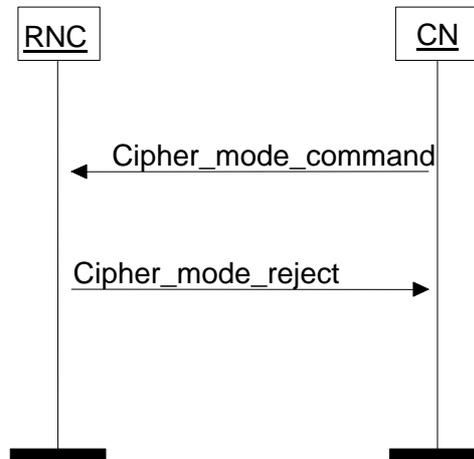
Figure ~~23~~[25](#). Cipher Mode Control procedure, unsuccessful case.
