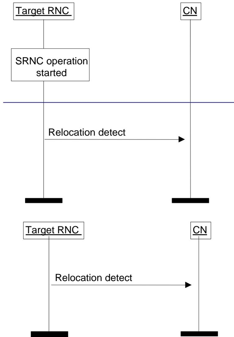
Figure 55. Relocation Detect procedure.
