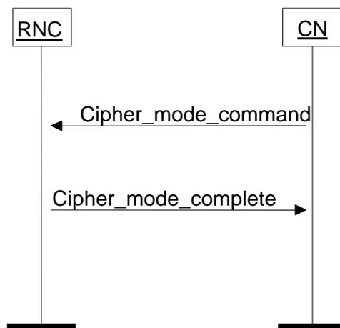
Figure ~~222224~~. Cipher Mode Control procedure, successful case.
