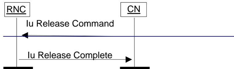
**Figure 16. Iu Release: successful handover or SRNS relocation.**
