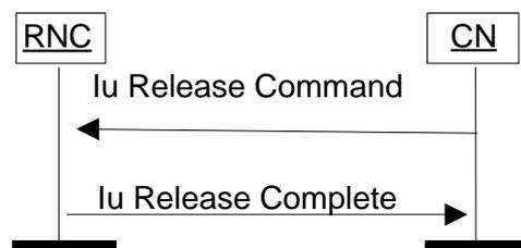
Figure ~~13~~14. Iu Release: ~~procedure~~Completion of transaction between UE and CN.
