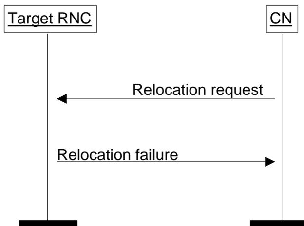
Figure 445. Relocation resource allocation failure.
